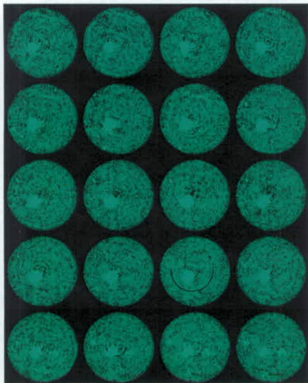
Figure 3. Synchrotron microtomography images taken 30 microns apart; the sequence is from left to right and top to bottom. The bright region strongly attenuates X-rays, so it may contain iron-based minerals such as pyrite and/or calcium minerals such as calcite.
