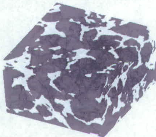
Figure 4. 3-D (1.1 mm each side) image of Berea sandstone. The pore space is white and the grains dark.
