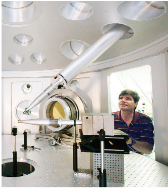
Using the Titan laser, researchers can explore high-energy-density physics issues, including the science of fast ignition for inertial confinement fusion.
