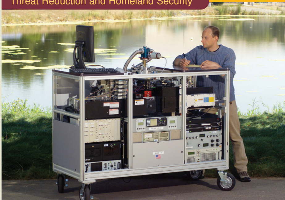
The Bioaerosol Mass Spectrometer, which won an R&D 100 Award, was connected to the air handling system in a major airport. The instrument demonstrated long-term, reliable performance.
