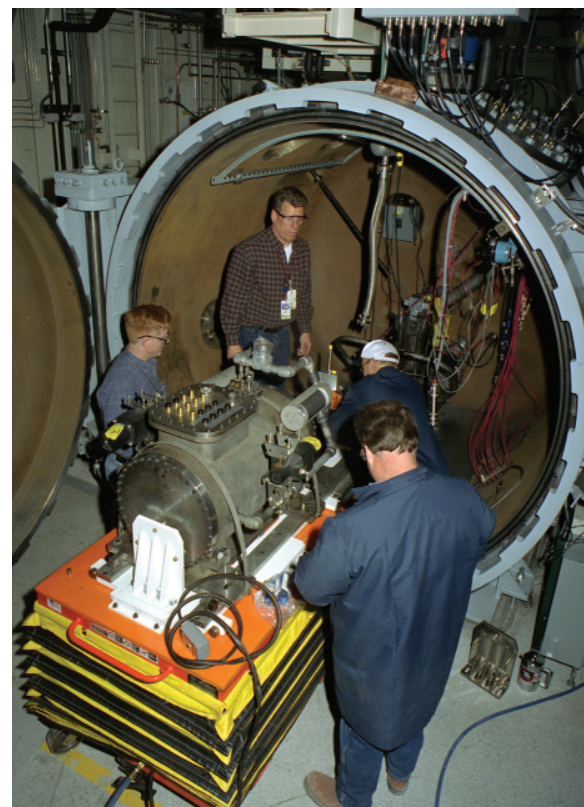
The target chamber at the JASPER facility is specially designed to ensure that plutonium dust or fragments are not released into the environment after an experiment.
