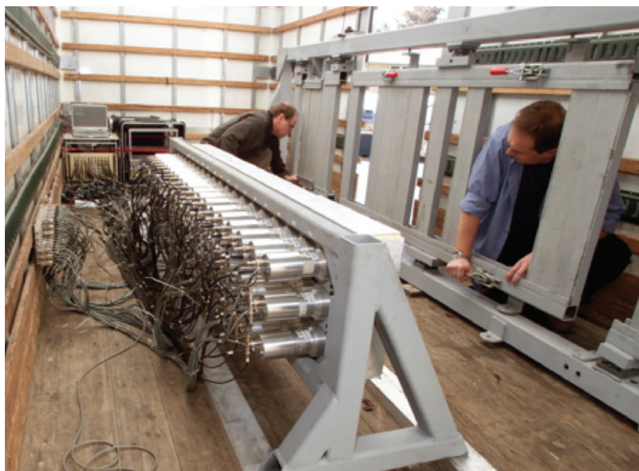
The sensitivity of the large-area, scintillator-based gamma-ray imaging detector makes it able to detect very small quantities of nuclear material.
