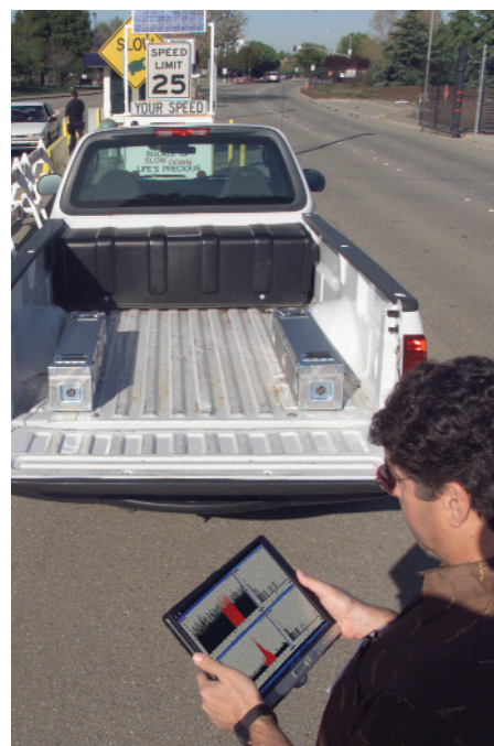
The Adaptable Radiation Area Monitor, which won an R&D 100 Award, has been commercialized and is in use at California borders.
