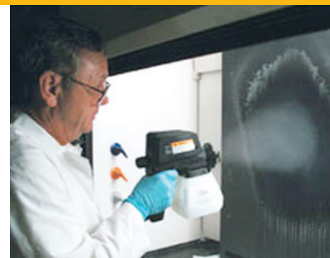
Biorestation after a terrorist attack could make use of L-Gel, a spray-on material for quickly and effectively destroying bioterror agents.
