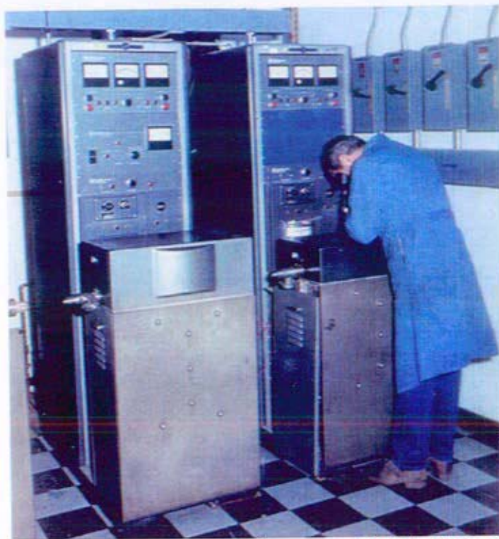
Figure 64: Photograph of two ultra-high vacuum aging furnaces at PMTI. Both are used strictly for refractory metals. They have Ta heating elements and can achieve temperatures as high as 2000 °C. Vacuum levels in the 10^{-8} to 10^{-9} torr levels can be maintained for long term anneals using metal to metal copper sealing rings in combination with sputter ion pumping systems. The heat zones are approximately 3-inches in diameter with a height of 10-inches.
