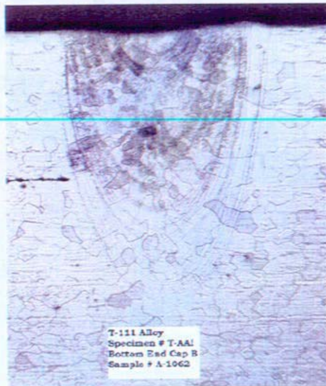
Figure 45: T-111, welded biaxial creep specimen. Tube is at the top left- end plug is bottom
