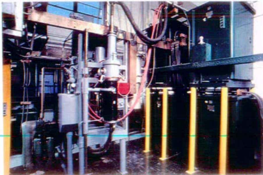
Figure 59: Leybold-Heraeus AC Arc Melter at PMTI. Maximum power input is 5000 amps. Maximum melt diameter for refractory ingots is ~4 inches.
