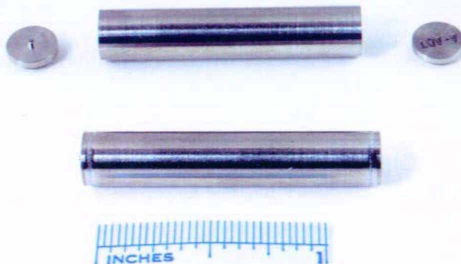
Figure 21: Top - Individual biaxial creep components. Bottom - Final welded biaxial creep specimen.
