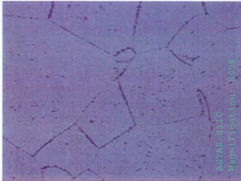
Figure 30: ASTAR-811C, 0.050-inch thick sheet, annealed at 1700 °C (Edge-longitudinal direction)
