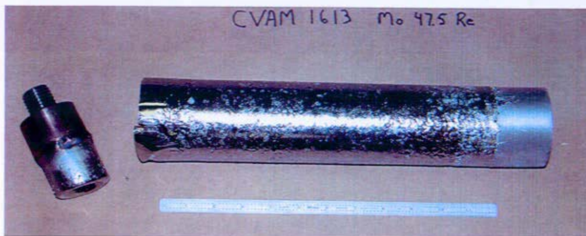
Figure 7: Final Melt 3-inch diameter Mo-47.5Re Ingot with starting pad still attached to the right. Remnant of the starting electrode is on the left.
