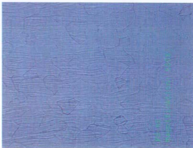
Figure 48: FS-85, 0.064-inch sheet, annealed, at 1400 °C (Edge –transverse direction)
