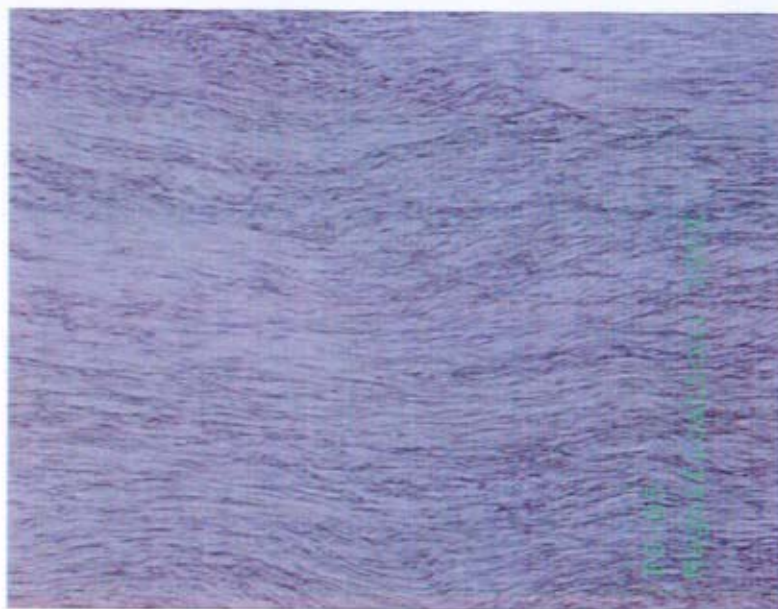
Figure 46: FS-85, 0.150-inch thick sheet, as-rolled condition. (Transverse direction)
