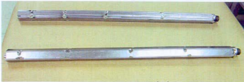
Figure 5: Two as-welded T-111 1 st melt sandwich electrodes. A pure Ta threaded adapter is welded to the top (right) of each electrode. The adapter is used to attach the electrode to the furnace and then serves as the transmission path for the melt current to the electrode.
