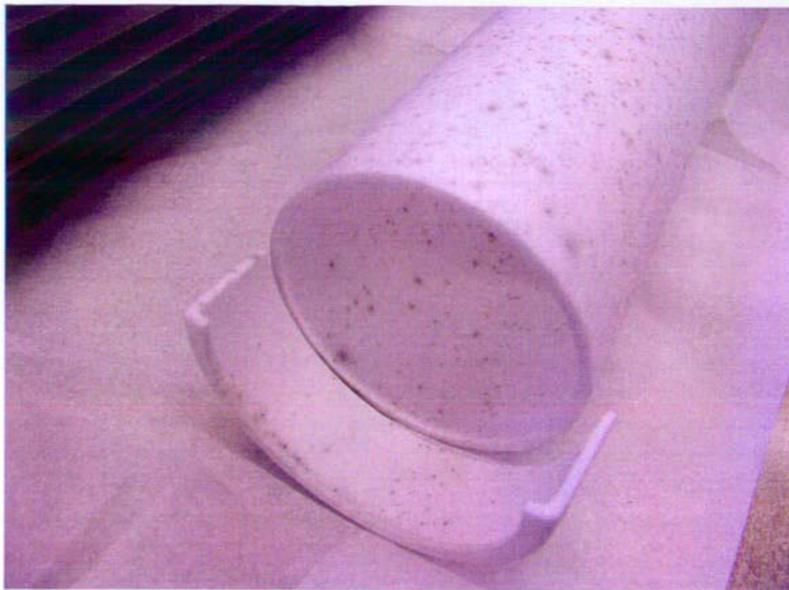
Figure 7: Contamination Found on Alumina Tube after Ta-10W Run
