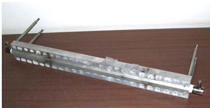
Fig. 6. Old heat exchanger for control system transistor cooling
