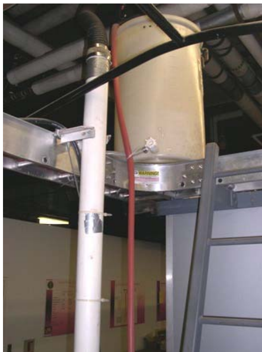
Fig. 12. Inlet pipe extension for stabilization of VOC concentration in the test points.
