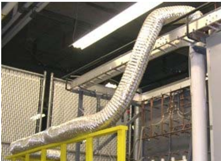
Fig. 12. Inlet pipe extension for stabilization of VOC concentration in the test points.
