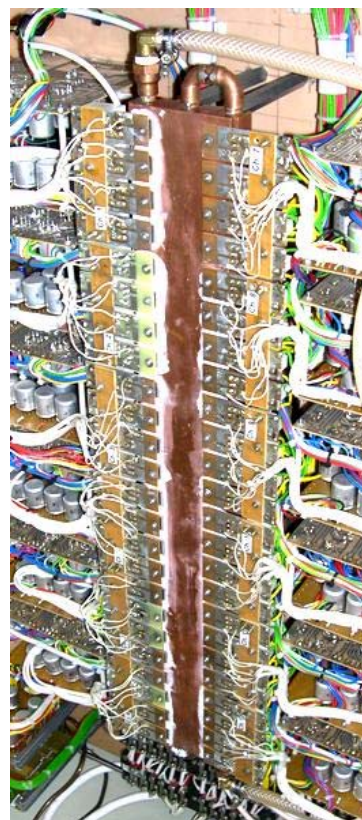
Fig. 7. New heat exchanger for transistor cooling in the control unit
