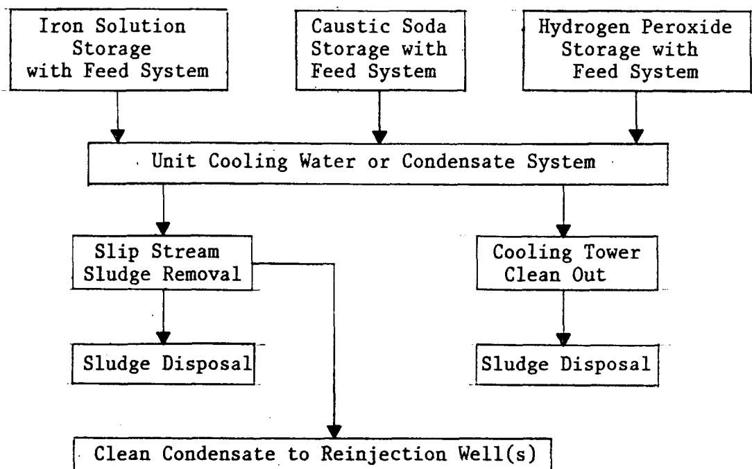
The chemical requirements for each unit are summarized in Table 3-6 and 3-7. The chemical quantities required are dependent on the units' capacity factor. Two capacity factor levels are presented: the 60 percent which plants are now operating, and the 70 percent which is anticipated to be the long range best capacity factor obtainable with this abatement system.
