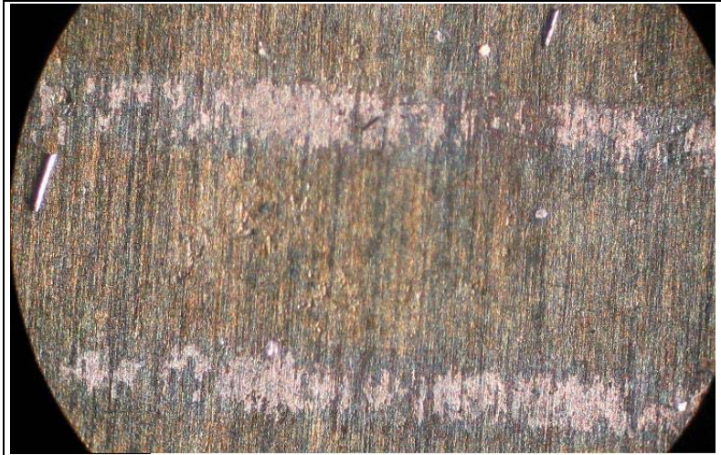
Figure 29 Oxidation in the Cathode Port showing imprint of bipolar plate flow field lands
