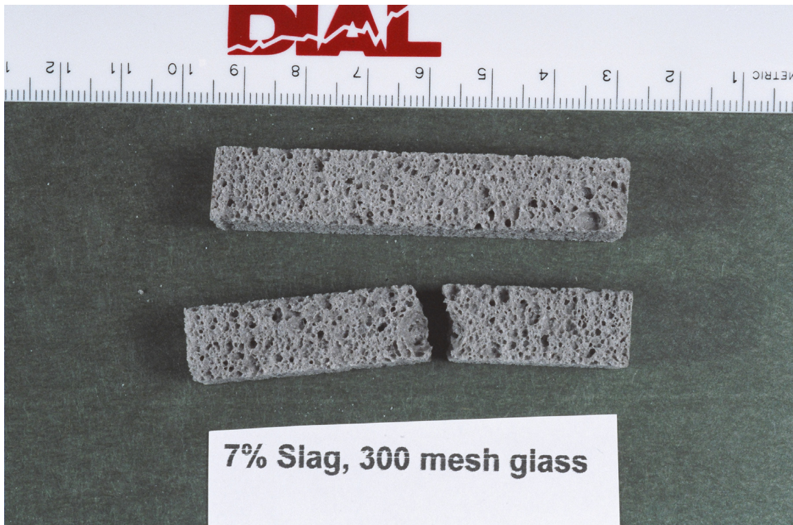
Figure 15. An unbroken test specimen for the four point bending test and a broken specimen. These specimens contained 7% Wabash slag, and the glass frit used was 300 series.
