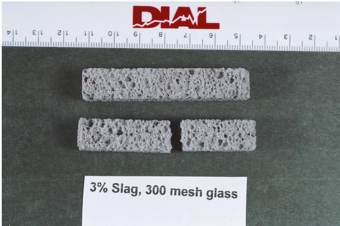
Figure 13. An unbroken test specimen for the four point bending test and a broken specimen. These specimens contained 3% Wabash slag, and 300 series glass frit was used. (300 series glass has a median particle diameter between 7 and 9 microns.) The scale at the top of the picture is graduated in centimeters and millimeters.
