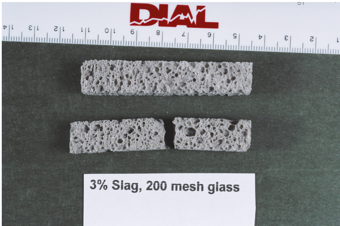
Figure 14. An unbroken test specimen for the four point bending test and a broken specimen. These specimens contained 3% Wabash slag, and the glass frit used was screened through a 200 series screen.
