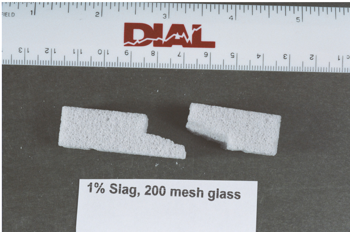
Figure 16. A broken specimen from the four point bending tests. This specimen exhibits an irregular fracture pattern that was observed on occasion.
