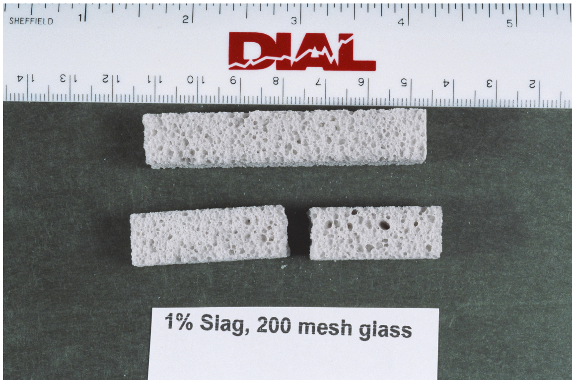
Figure 12. An unbroken test specimen for the four point bending test and a broken specimen. These specimens contained 1% Wabash slag, and was made using 200 series glass, with a median particle diameter between 9 and 11 microns.
