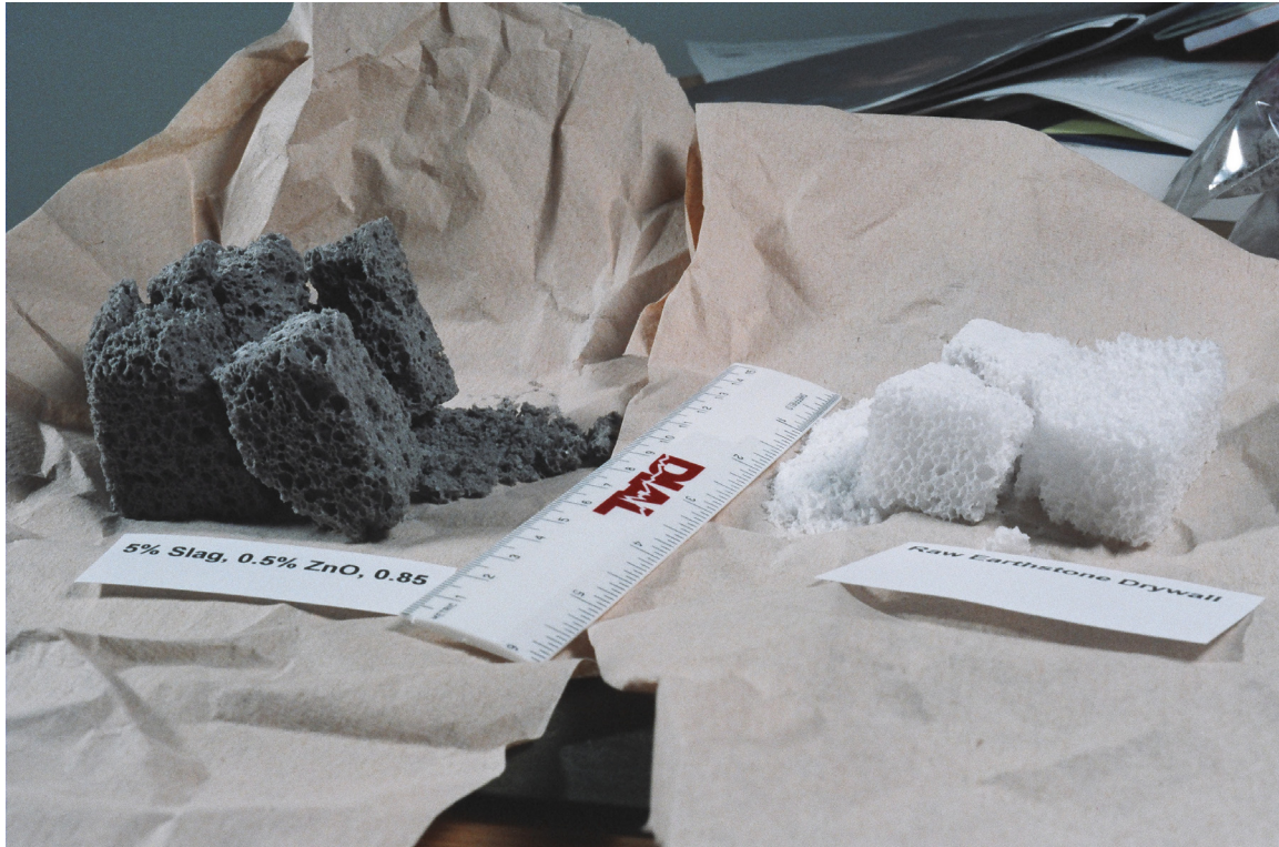
Figure 17. Fractured samples from compressive (crushing) strength tests. On the left is the foamed glass sample with 5.0% Wabash slag, 0.5% zinc oxide, and 0.85% calcium carbonate. On the right is the sample of the baseline drywall product. These test specimens were originally 50.8×50.8×50.8 mm (2×2×2 inch) cubes.
