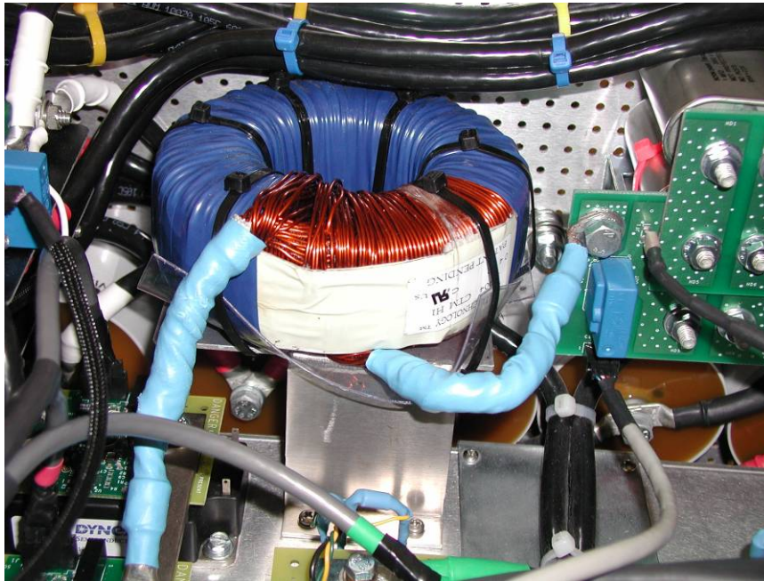
Figure C4. Improved Resonant Inductor Installed In ETM Prototype.
