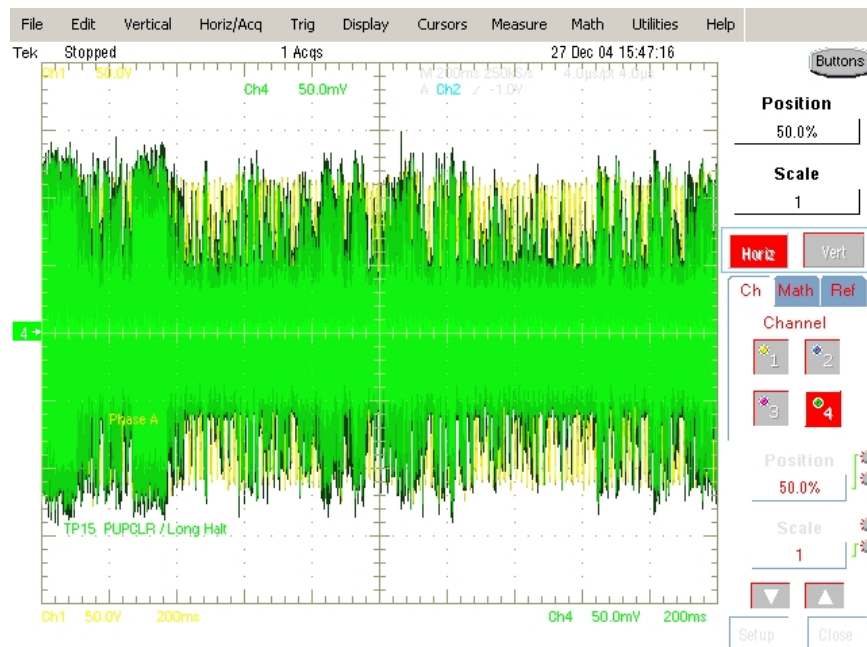
Figure C8. Resonant Signals VRC (green) and IRMAG_SIGN (yellow).
