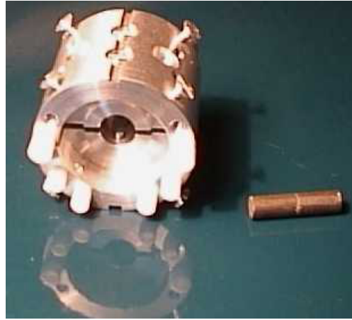
Figure B.2: Compass holder (top and bottom halves), and glued Nd-Fe-B magnets used as the needle.
