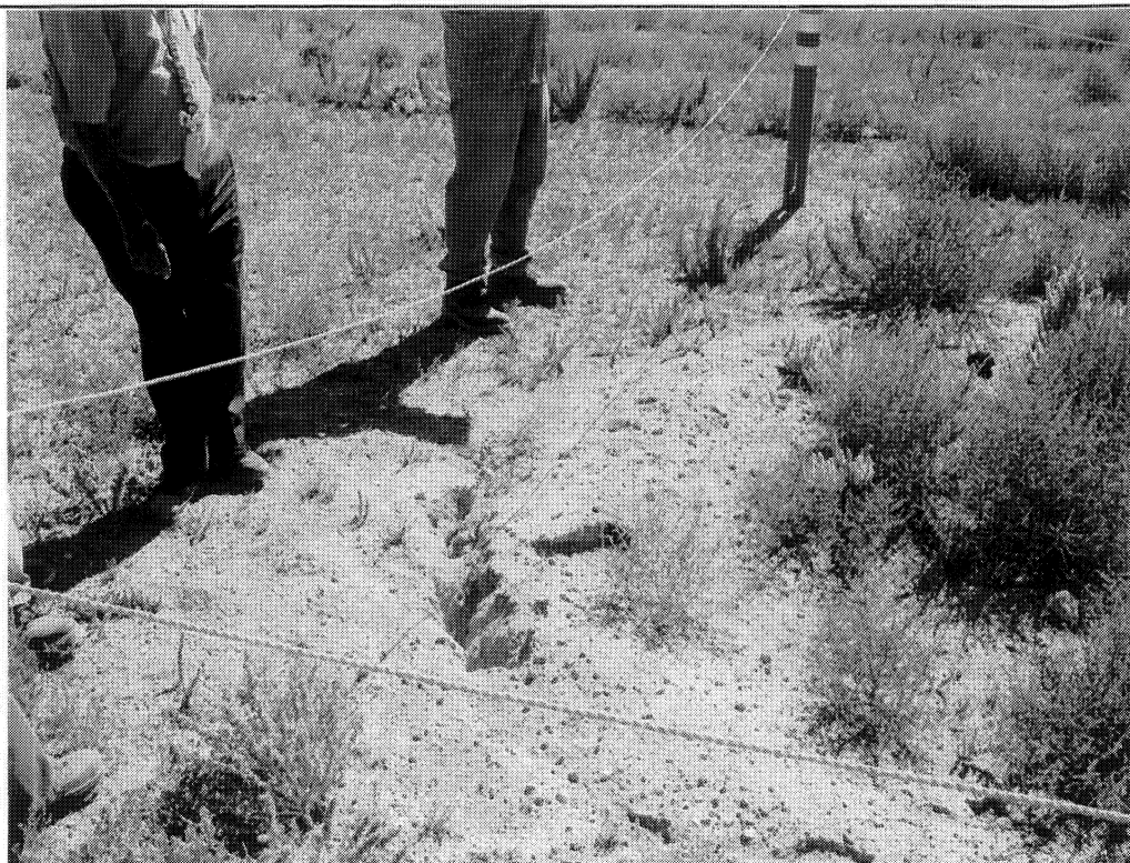
11. Subsidence area along southeast side of cover.
