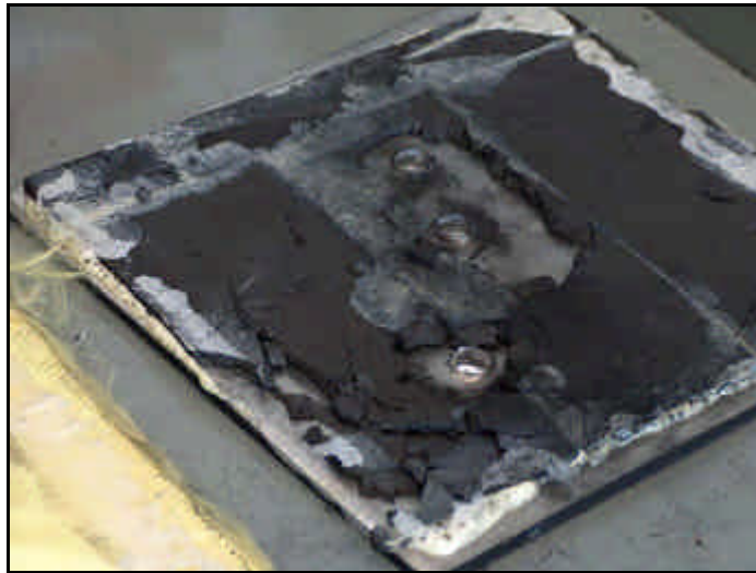
Figure 36. The back view of Carbon Foam Sample #1's first layer of carbon foam.
