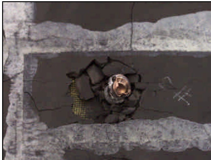
Figure 23. Damage of the 35 lb/ft 3 layer of carbon foam to the 357 Magnum round in Carbon Foam Sample #3.
