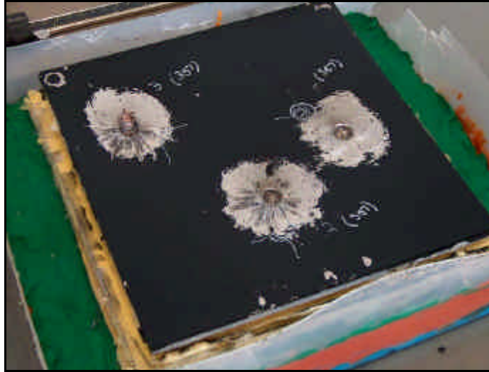
Figure 33. Points of contact on the Control Sample by the 357 Magnum rounds.
