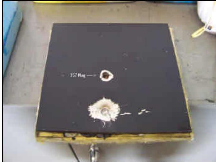
Figure 22. Point of entry for the 357 Magnum round on Carbon Foam Sample #3
