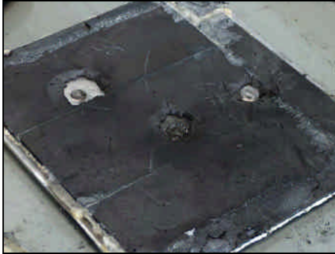
Figure 29. 35 lb/ft 3 carbon foam layer reaction on Carbon Foam Sample #1 (viewed from behind).
