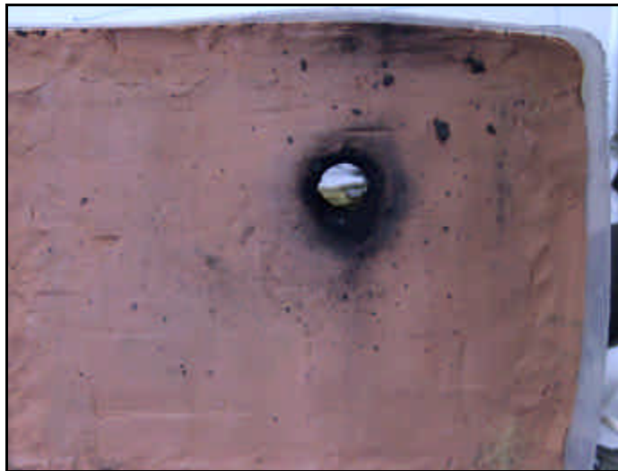
Figure 27. Penetration of the AR-15 round through the clay backing for Carbon Foam Sample #1.
