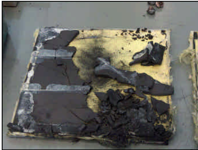
Figure 38. The second layer of carbon foam reaction on Carbon Foam Sample #2
