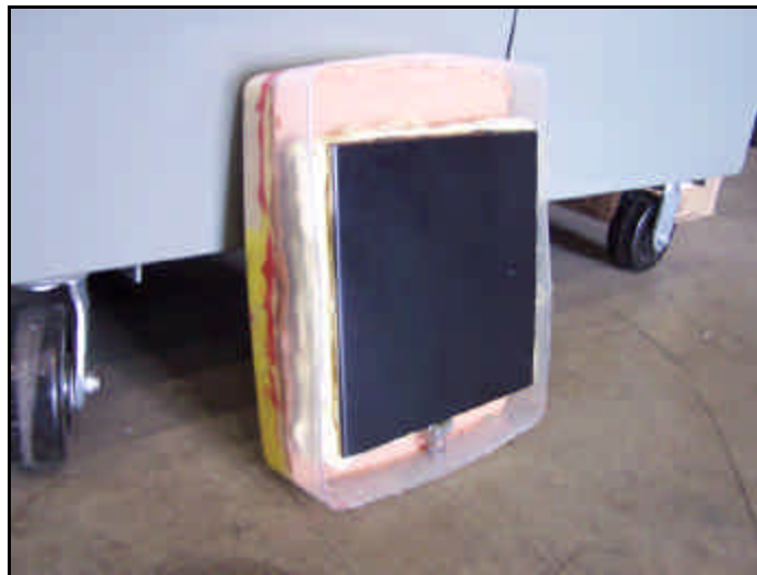
Figure 18. Orientation of armor sample and clay backing box
