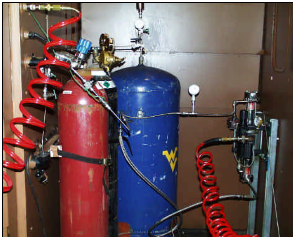
Figure 41. The blue tank in the rear is a holding tank to allow vented gas to be temporarily stored and slowly vented.
