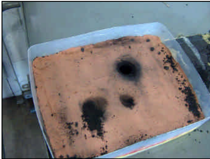
Figure 32. Blunt trauma reaction to 357 Magnum rounds on Carbon Foam Sample #1.
