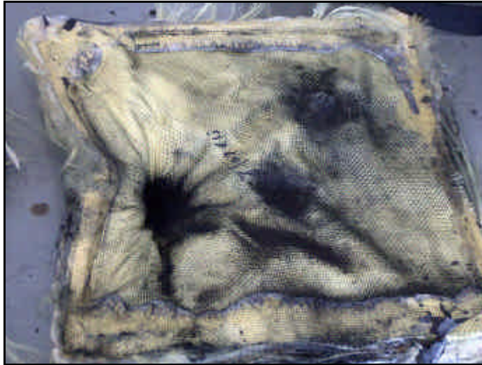
Figure 30. Reaction of the 8 layer Kevlar section on Carbon Foam Sample #1.
