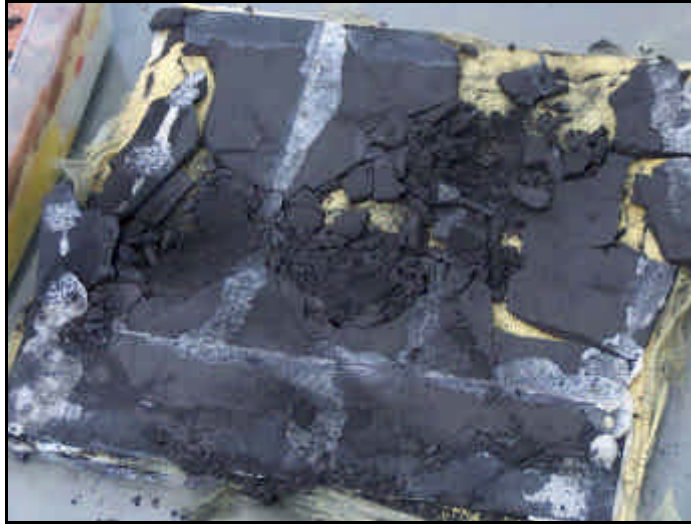
Figure 31. Reaction of the middle layer of carbon foam on Carbon Foam Sample #1.
