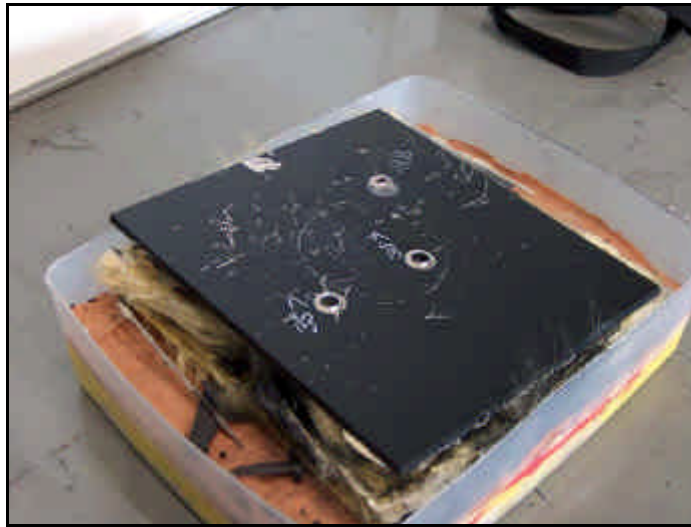
Figure 28. Carbon Foam Sample #1 after being tested with 357 Magnum rounds and AR-15 round.
