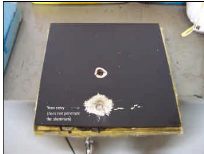
Figure 19. Point of entry for the 9mm round into Carbon Foam Sample #3
