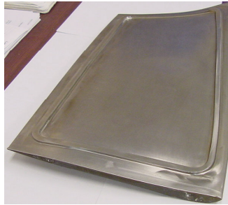
Figure 41 - 33.5" Advanced Aero Design: Caul sheet tool
