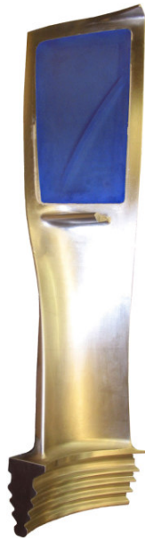
Figure 43 - 33.5" Advanced Aero Design: One Outboard Pocket with One Rib
