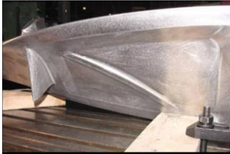
Figure 14 - Machined Pocket: 33.5" Advanced Aerodynamic Design Hybrid LSB
