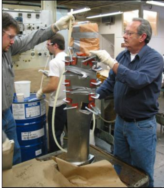
Figure 18 - Bucket Standing Upward during the Hybrifil Filling Operation
