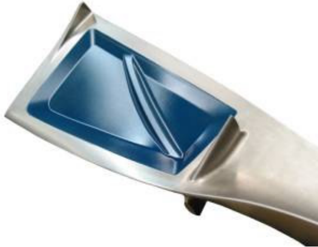
Figure 15 - Surface of Primed Pocket (Prior to Hybrifil Filling)
