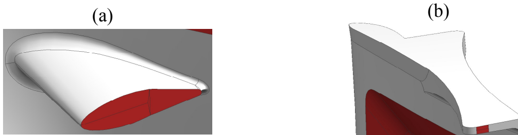
Figure 2 - 54” Steel-Hybrid: Design Features (a) Winglet; (b) Snubber Cover
