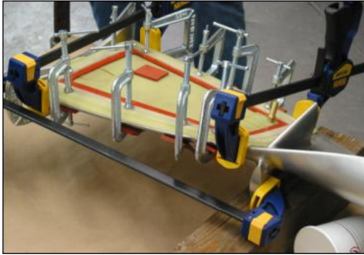
Figure 17 - Caul Sheet Partially Clamped on the Bucket
