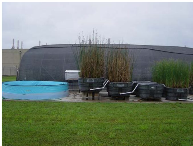
Figure 2. Pilot constructed wetland system at Clemson University for treating FGD wastewater.
