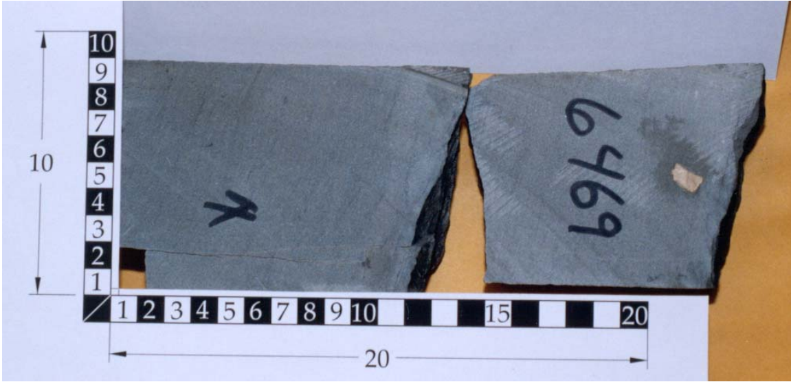
Figure B43. RB E 01 at 6,469 ft showing near-vertical fracture in lower left portion of photograph (image by Craig Shirley).
