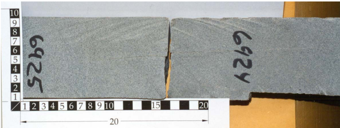
Figure B44. RB E 01 at 6,924 to 6,925 with high-angle fracture (image by Craig Shirley).
