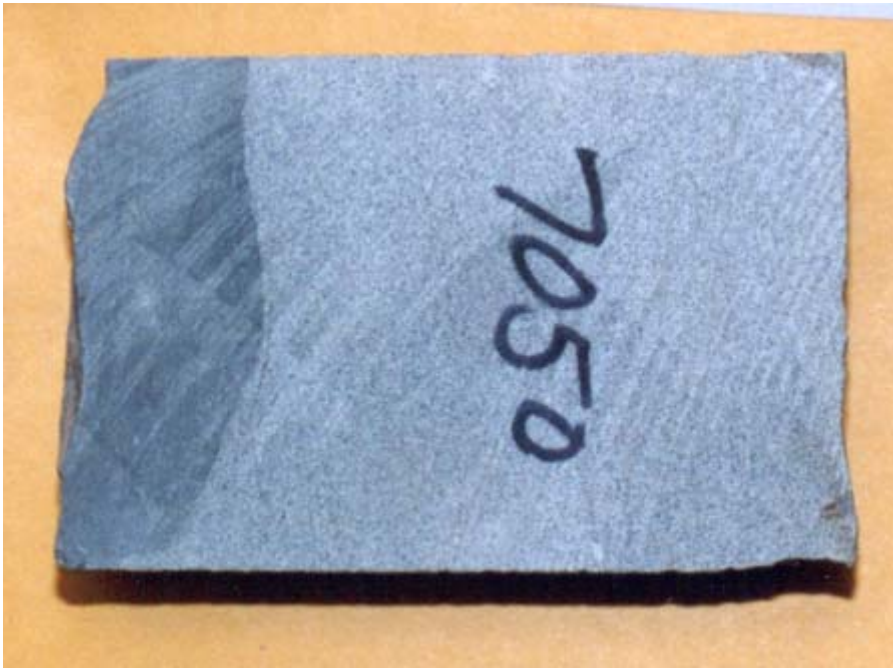
Figure B33. RB U-2 core at depth of 7,050 ft showing visible contact (image by Craig Shirley).
