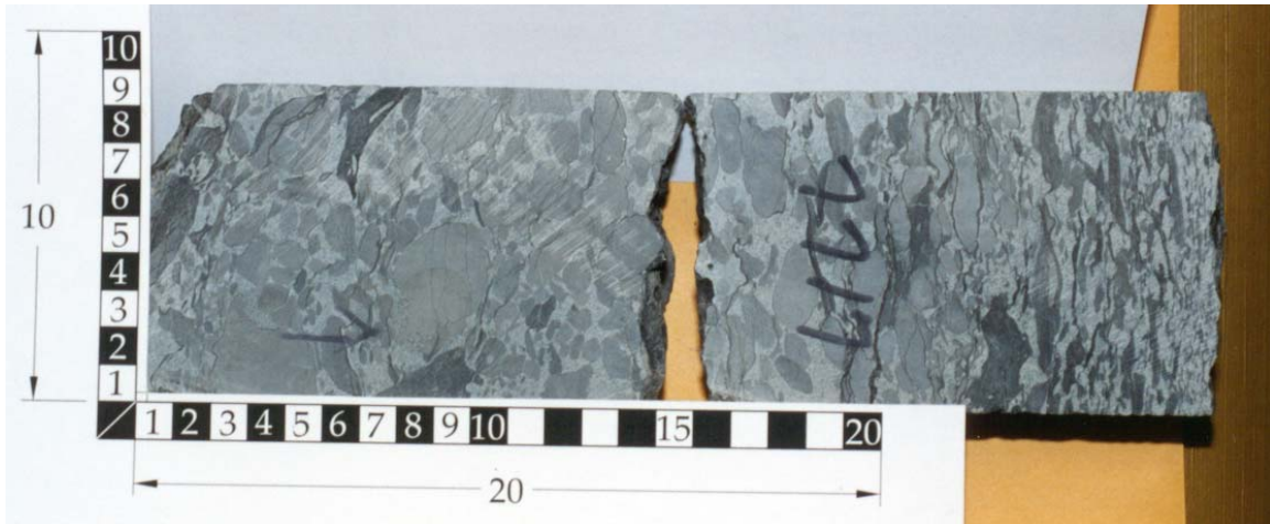
Figure B37. RB U-2 core at 7,717 to 7,718 ft with numerous clasts and laminae (image by Craig Shirley).
