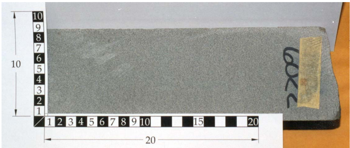
Figure B42. RB E 01 at 6,022 ft core parting at subtle shift in grain size (image by Craig Shirley).
