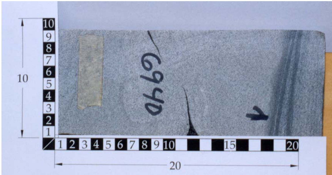
Figure B45. RB E 01 at 6,940 ft showing carbonaceous stringer and laminae (image by Craig Shirley).
