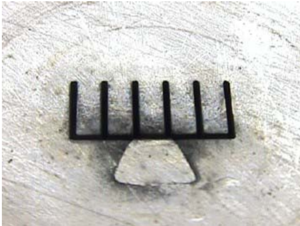
Figure 27. Close-up view of the microchannels cut in the target block.
