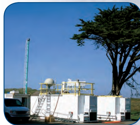
State-of-the-art active and passive remote sensors measured the detailed microphysical structure of marine stratus clouds at the AMF deployment site, about 1 mile from the ocean at Point Reyes National Seashore.
