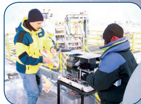
The 183 GHz radiometer, protected inside an insulated enclosure (inset), is installed on the roof of the primary instrument shelter at Barrow. To prevent snow from accumulating on the mylar window, a blower mounted beneath the radiometer directs air through a duct to a standard Y-shaped fitting mounted on top of the radiometer.
