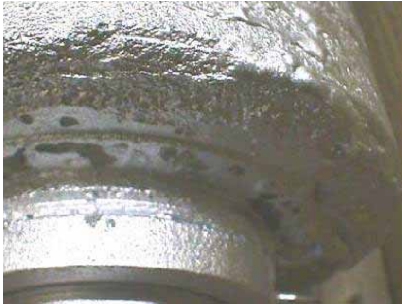
Figure 5: Close up of dross formation
