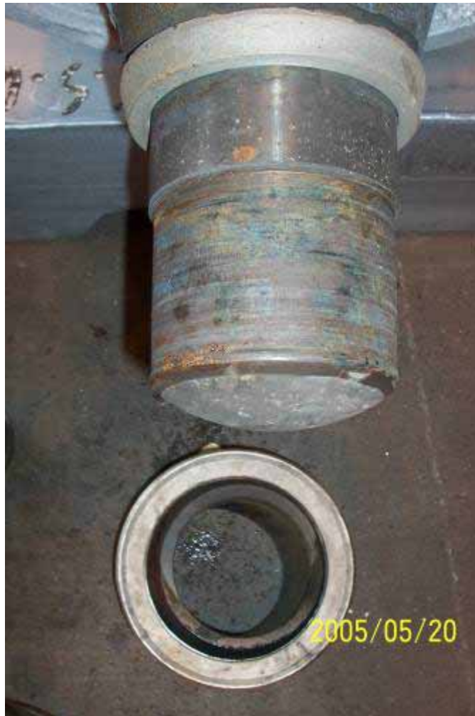
Figure 119: Shaft/bearing assembly after trial at steel partner A
