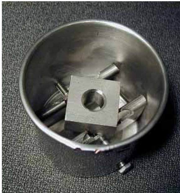
Figure 55: Stainless Steel Strut Channel and Seat Bolted into Specimen Cup
