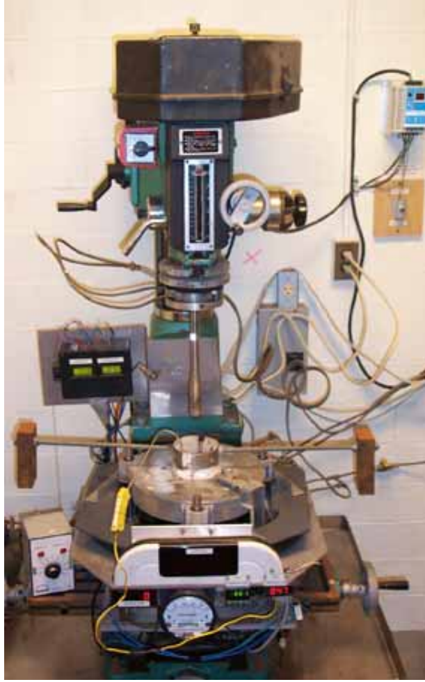
Figure 56: WVU's Small-Scale Zinc-Pot Bearing Materials Tester
