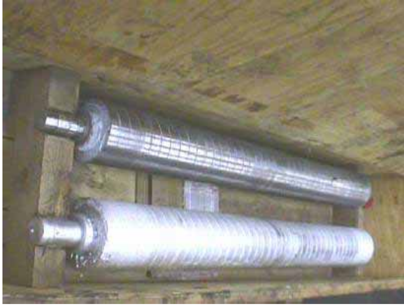
Figure 3: Stabilizer rolls from steel partner B
