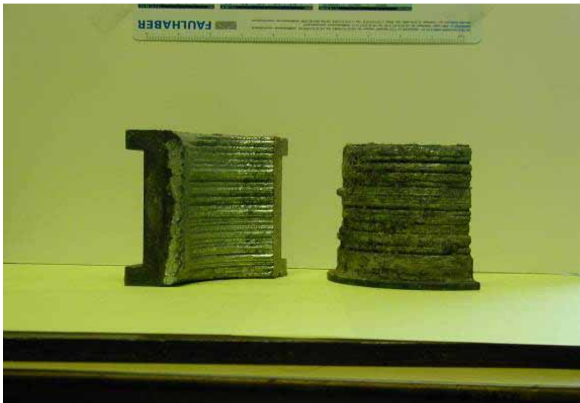
Figure 121: Stellite 6 bearings after service.
