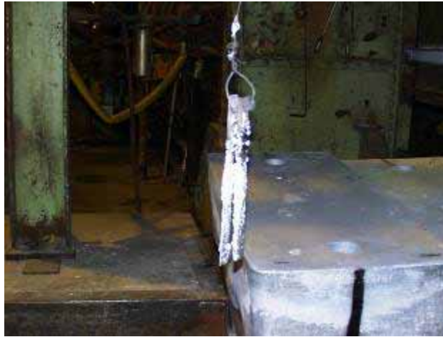
Figure 47: Static corrosion specimens coming out of the industrial bath
