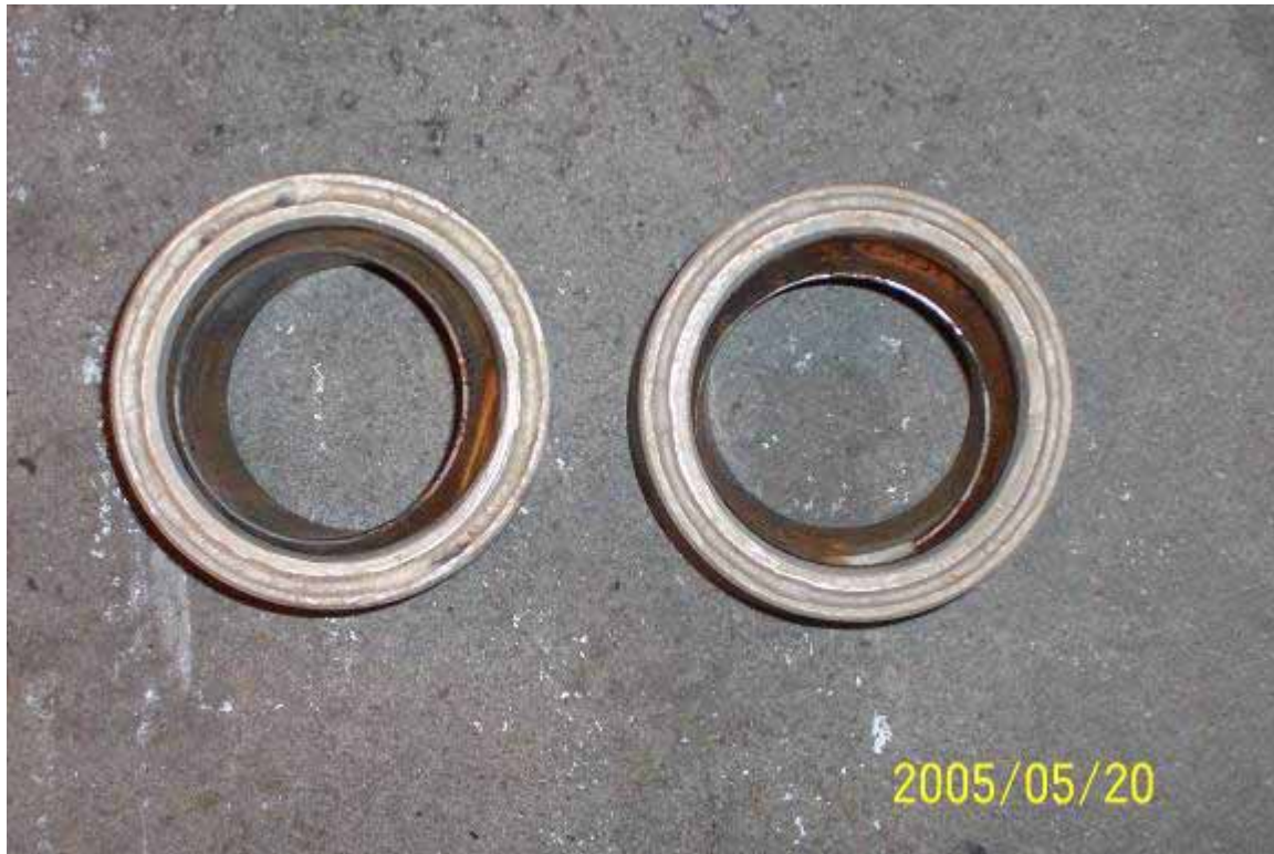
Figure 120: 2012 XT Stabilizer roll bearing after 16 days trial at steel partner A
