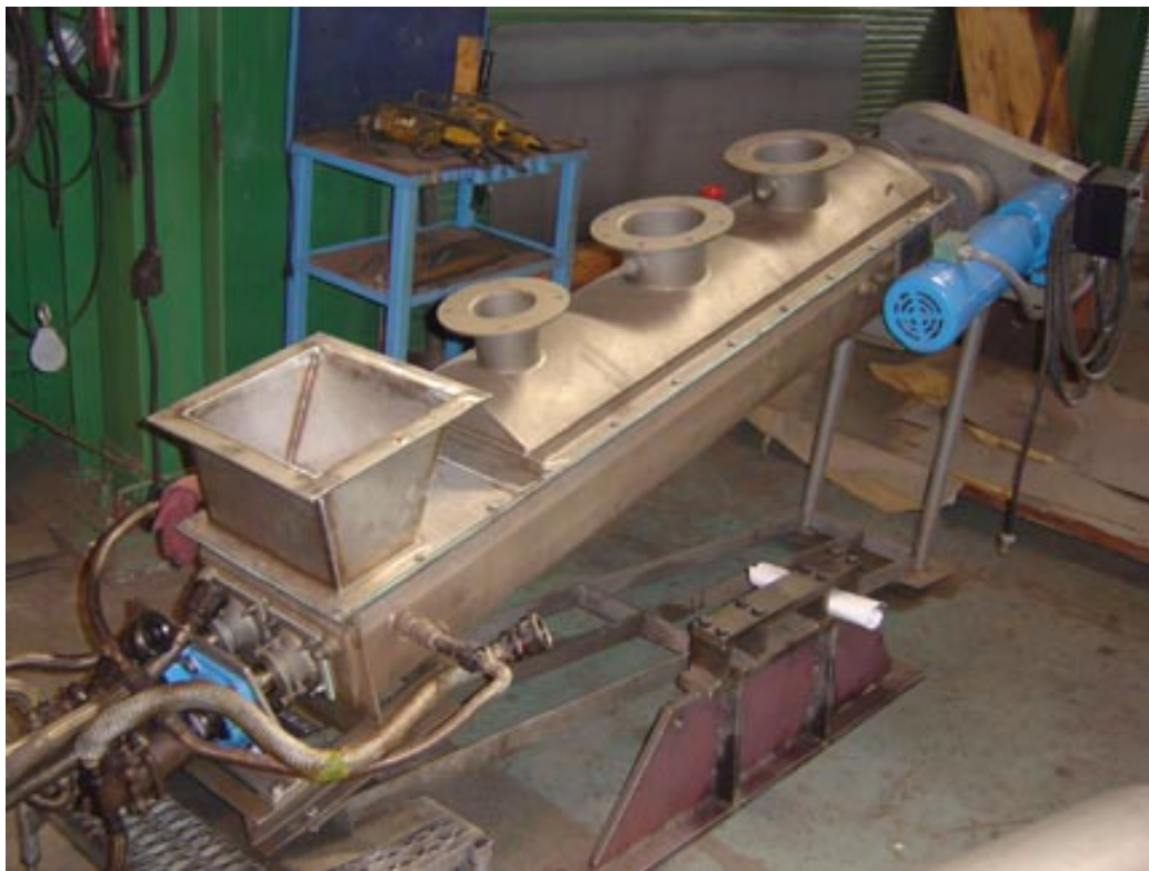
Figure 1. Therma-flite's bench-scale screw conveyor test unit
