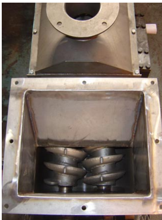
Figure 2. Feed inlet of Therma-flite's bench-scale test unit
