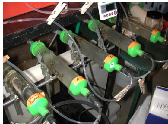
Examples of the acrylic minipipes used in the tests. The pipe with clear water on left is an untreated control, whereas water in other pipes has a grayish color due to presence of suspended bacteria during treatment. Mussels are visible attached to walls of pipe.
