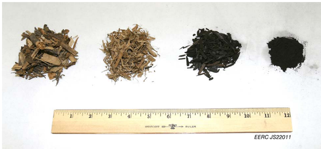
Figure 18. Comparison of milling tests performed on the raw unprocessed UWW (-1 in.), as compared to the CSR processed UWW obtained from Test 6.
