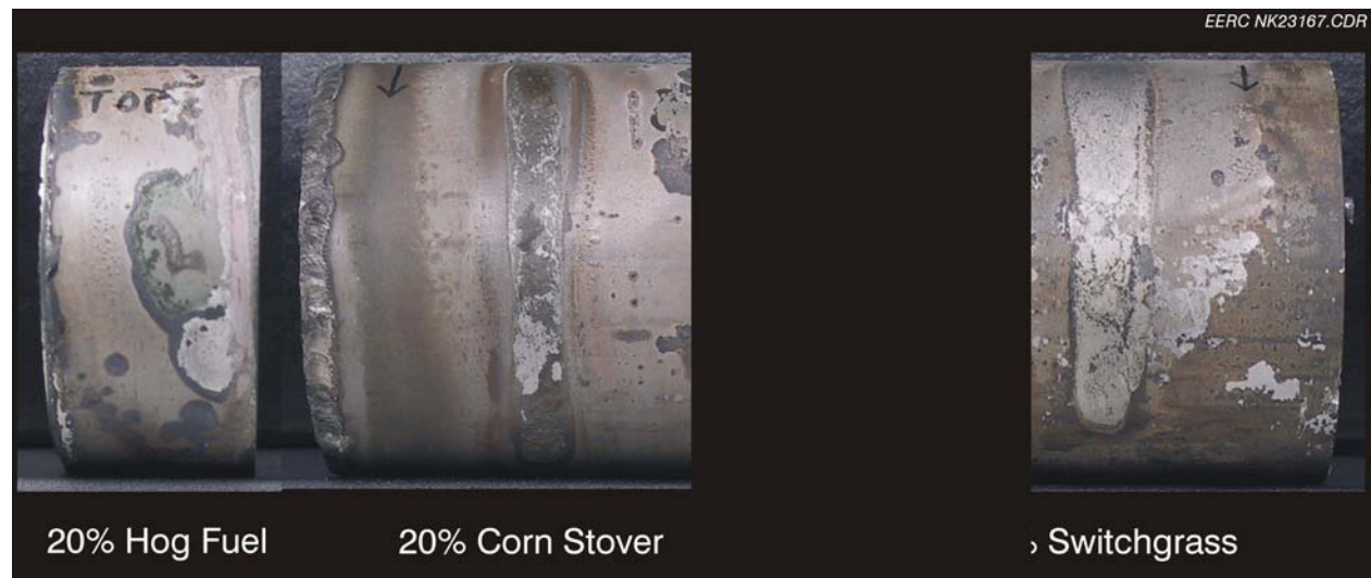
Figure 2. The surfaces of the MA956 tube sections after flowing slag corrosion testing in the DSAF.
