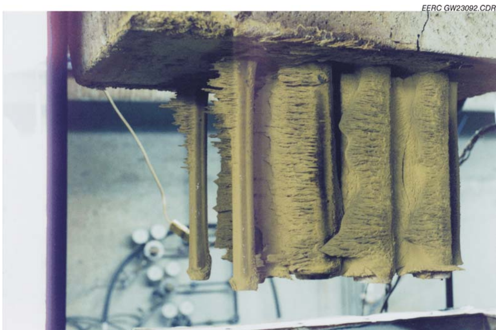
Figure 12. Photograph of ash deposits on the surface of the tubes following Test XCEL2.
