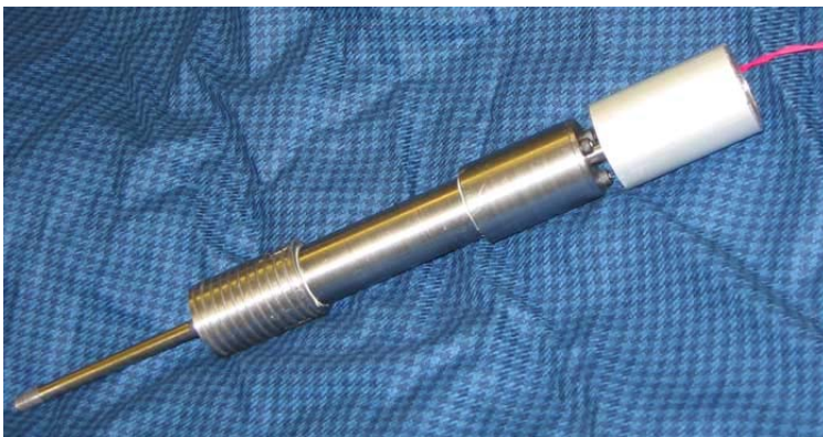
Figure 3.3.5: Low-carbon steel housing of the double-shafted MR damper
