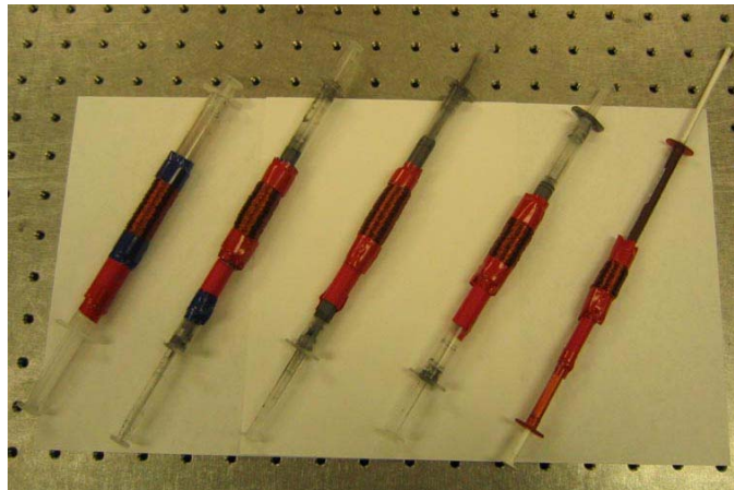
Figure 3.3.6: Syringe dampers with varying housing and valve dimensions
