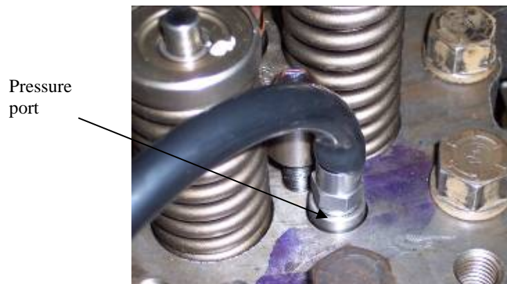
Figure 8. Top view of the cylinder head with pressure sensor port
