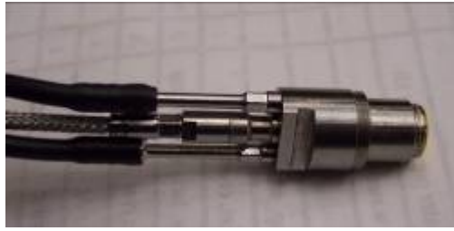
Figure 6. Kistler type 6067C pressure sensor
