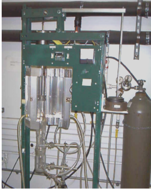
Figure 7. Photograph of the new apparatus for aging specimens under stress. The hinged furnace is open, exposing the heating lamps and tensile loading fixture. Part of the linkage rod, L, outside the furnace and atmosphere chamber is visible.
