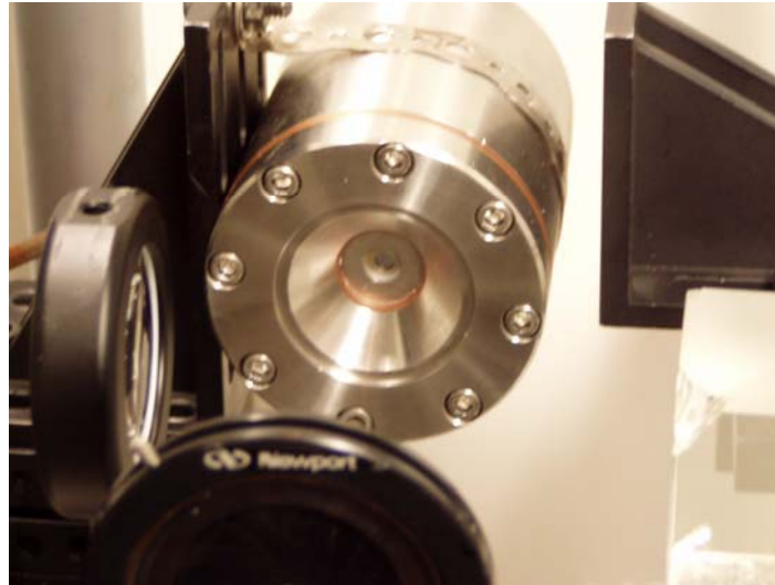
Fig.20. Close-up view of the experimental SiC chip mounted in the high pressure cell.
