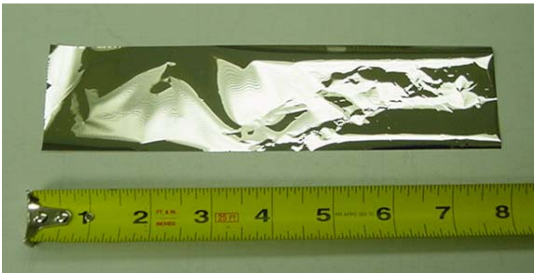
Figure 2. Rectangular membrane cut from 12-inch sample.
