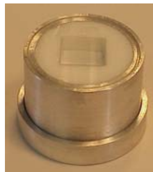
Figure 6. Photograph of a packaged \text{LaBr}_3 scintillator.
