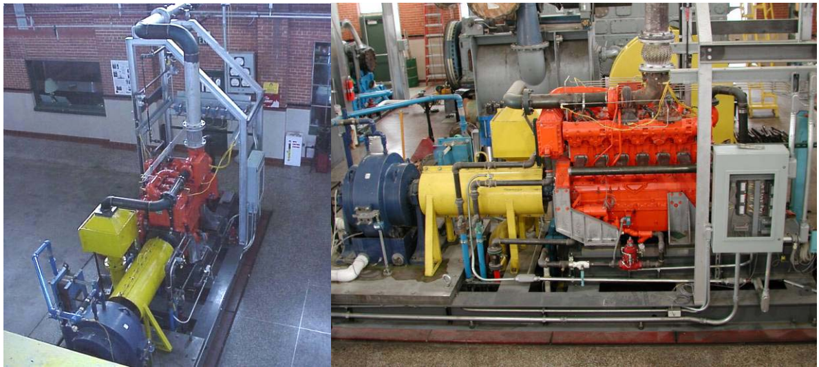
Figure 6-1: Waukesha VGF-F18GL Installed at the Large Bore Engine Test Bed at Colorado State University
