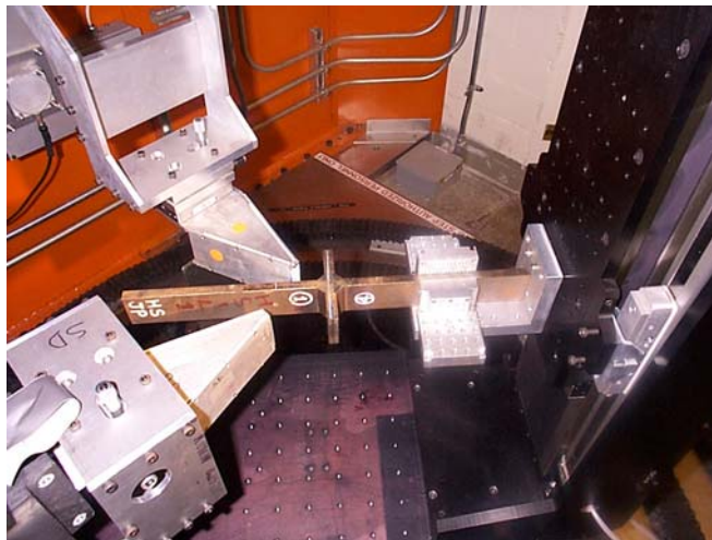
Fig. 64: Neutron scattering experiments were carried out on the new Neutron Residual Stress Facility (NRSF2) at ORNL.
