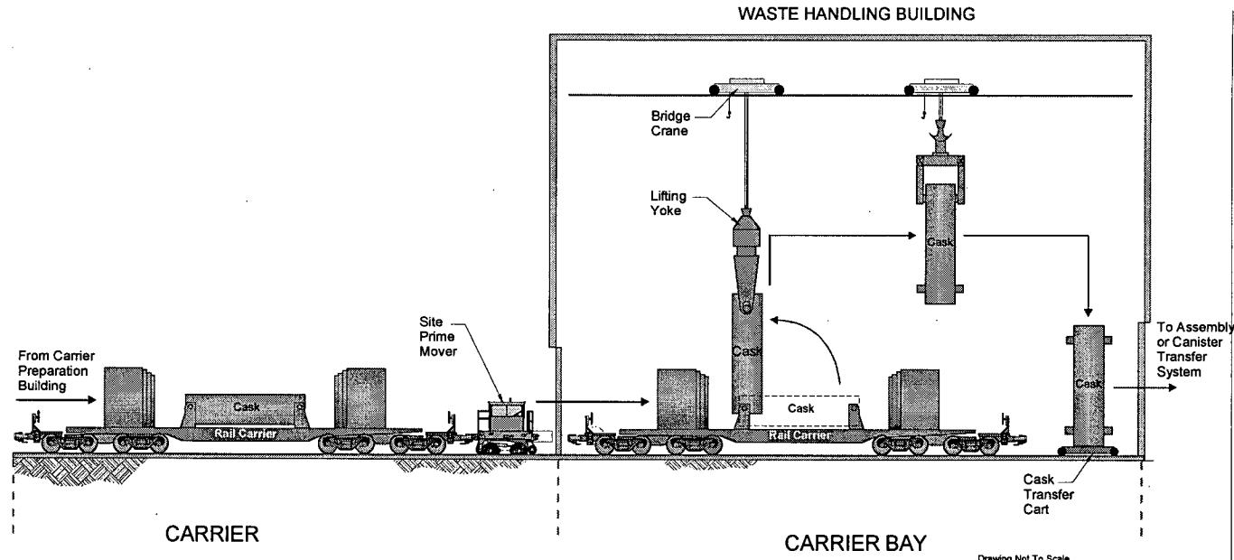
Figure 1. Carrier/Cask Handling System
