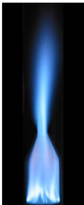
FIGURE 42: PHOTOGRAPH OF THERMJET BURNER FLAME WITH RETROFITTED QUARTZ NOZZLE
