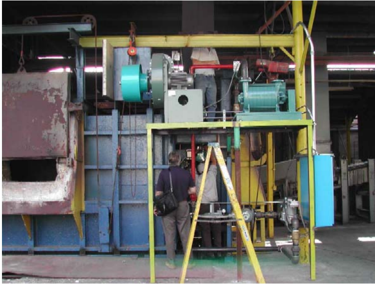
FIGURE 62 PRIMARY BLOWER (LEFT) AND SECONDARY BLOWER (RIGHT) USED TO PROVIDE THE PRIMARY COMBUSTION AIR AND SECONDARY INJECTION AIR TO THE BURNERS
