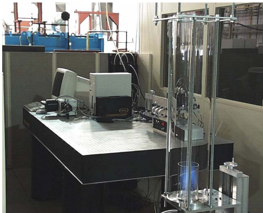
FIGURE 3 NOZZLE-MIXED BURNER, CONTROL SYSTEM, AND OPTICAL SENSOR
