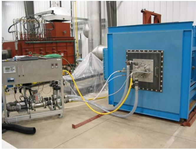
FIGURE 10 SOCS/FLEX-FLAME BURNER MOUNTED ON FURNACE AND CONNECTED TO AIR/GAS DELIVERY SKID
