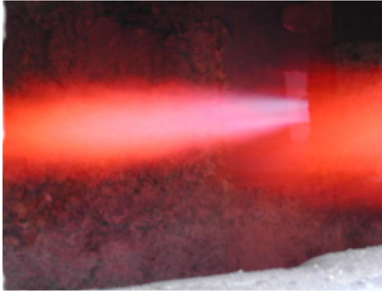
FIGURE 64 NEWLY INSTALLED HIGH-MOMENTUM THERMJET BURNERS FIRING AT 70% CAPACITY
