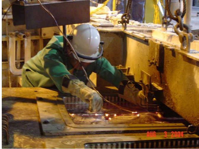
Fig. 4.2. A researcher placing a temperature jig into the molten aluminum in a DC casting mold at Aleris International's Newport, Kentucky, plant.
