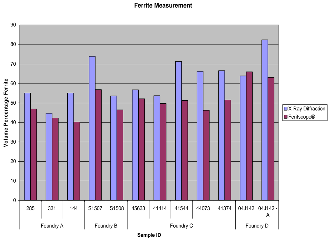
Figure 106: Comparison of Volume Percentage of Ferrite from Feritscope® and X-Ray Diffraction
