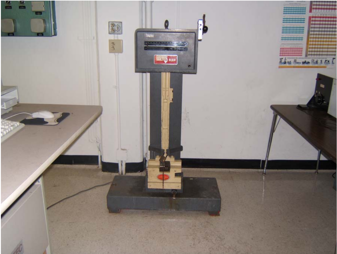
Figure 9: Charpy Impact Testing Machine
