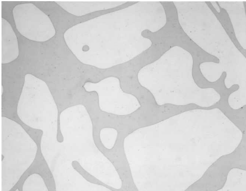
Figure 36. Microstructure of CD3-A-2, NaOH, 400x
