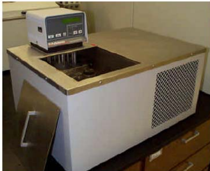
Figure 4-2. CPT Test Apparatus
