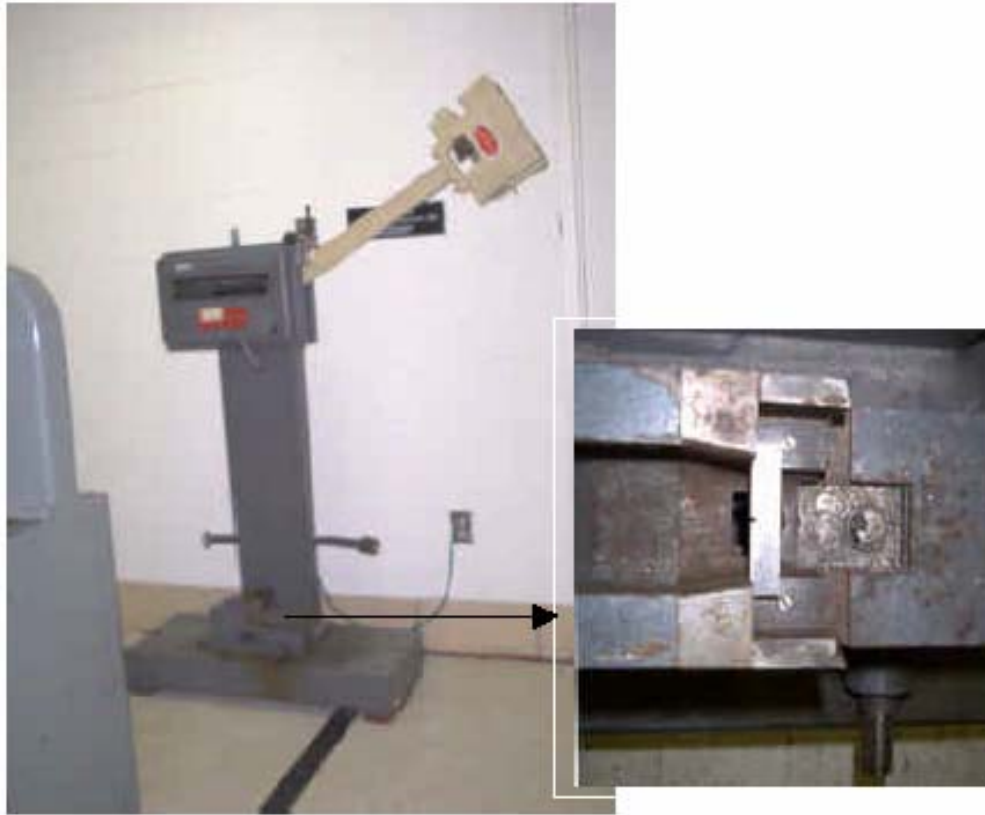
Figure 4-7 Charpy Test Apparatus Setup
