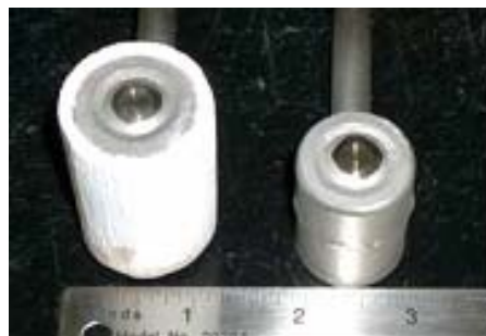
Figure 5.1.y. Air/N 2 -assist atomizing nozzles that include a separate water cooling jacket. The white jacket is added ceramic insulation.
