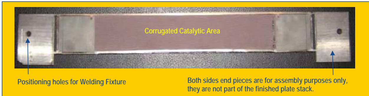
Figure 5.2.13. SP-2 plate with added frame.
