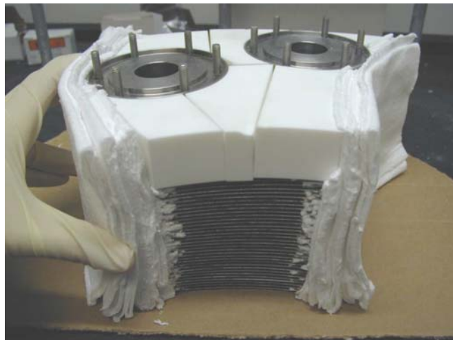
Figure 5.1.b. Blank plate stack with Fiberfrax insulation.
