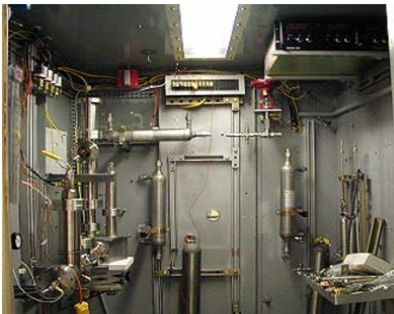
Figure 5.1.e. Lab set-up with heat exchangers, back pressure regulators, reactor, etc.
