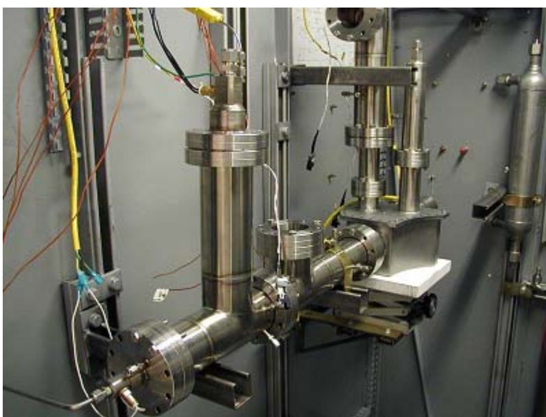
Figure 5.1.f. Lab set-up with reactor, thermocouples, injectors, and heaters.
