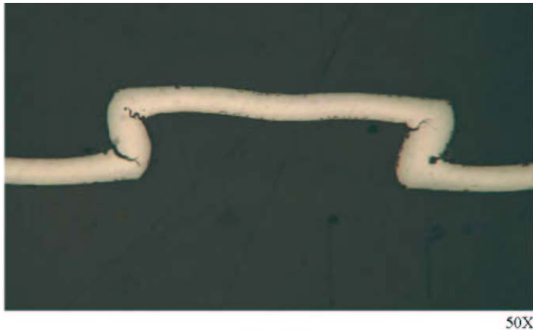
Figure 5.0.h. Cross-sectional view of crushed foil.
