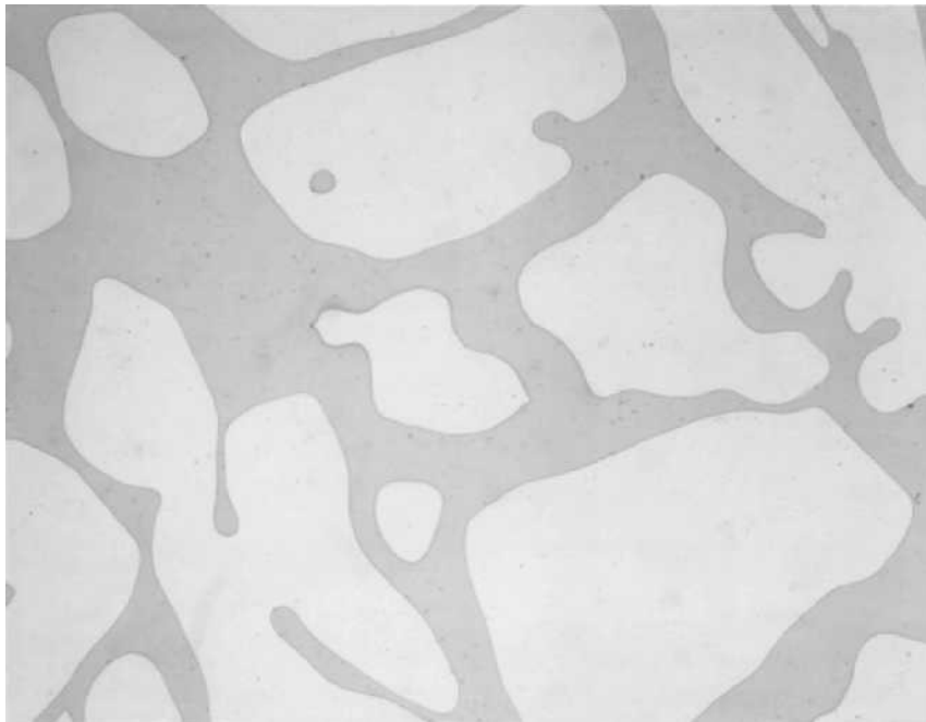
Figure 36. Microstructure of CD3-A-2, NaOH, 400x
