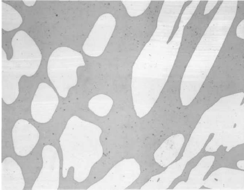
Figure 35. Microstructure of 42R-A-1, NaOH, 400x
