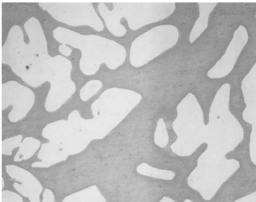
Figure 59. Microstructure of 42R-G-2, NaOH, 400x
