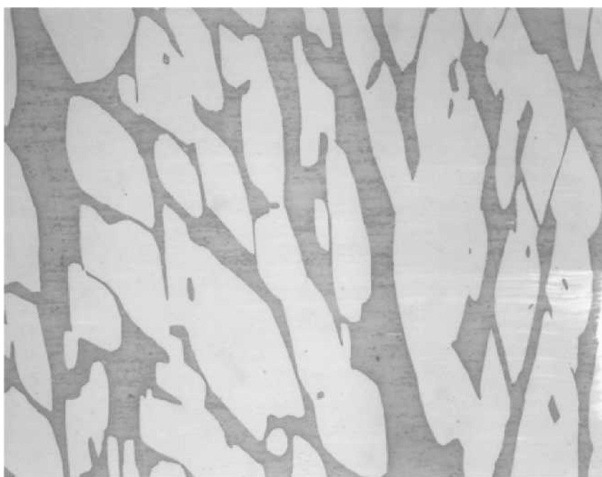
Figure 60. Microstructure of CD3-G-2, NaOH, 400x
