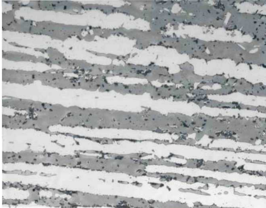
Figure 53. Microstructure of 2205-F-3, NaOH, 400x
