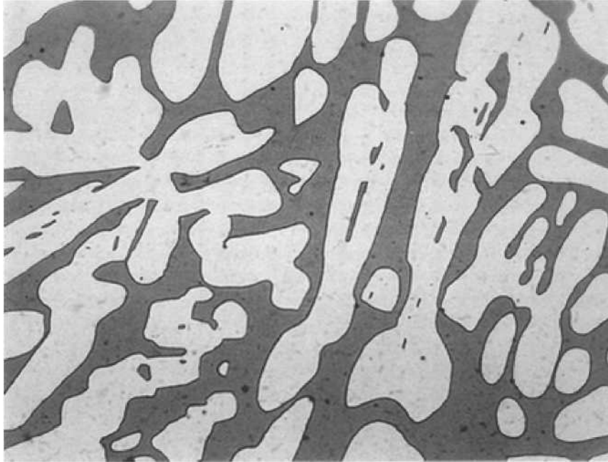
Figure 70. Microstructure of 41NCC-A-1, NaOH, 400x, Participant 5
