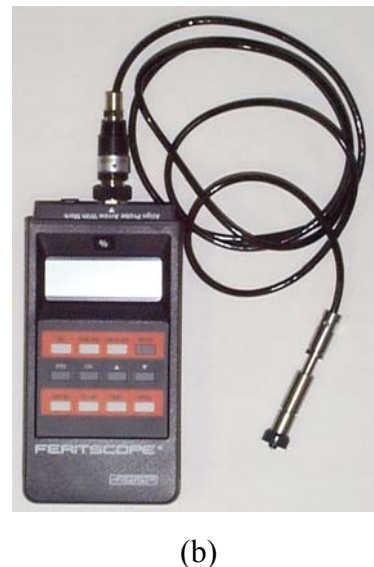
Figure 3-23. Ferrite Measurement with Single and Two-Pole Probes (a), and Feritscope® (b) [123]
