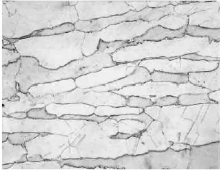
Figure 5-35. Microstructure of Wrought Alloy 2507, Oxalic, 400X
