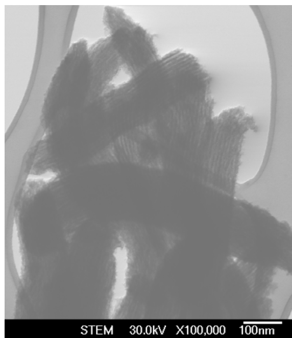
Figure 1. A cluster of defective SBA particles. These particles have pore diameters of about 10 nm, and the particles tend to be 500-1000 nm in length, appreciably shorter than particles of well-ordered SBA-15 [5].
