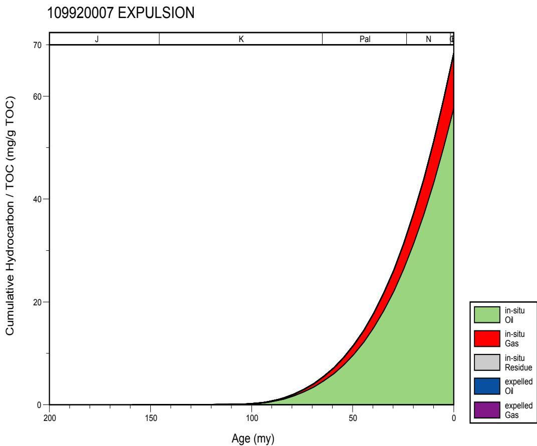
**Figure 64. Hydrocarbon expulsion plot for well 109920007, Manila Subbasin.**
