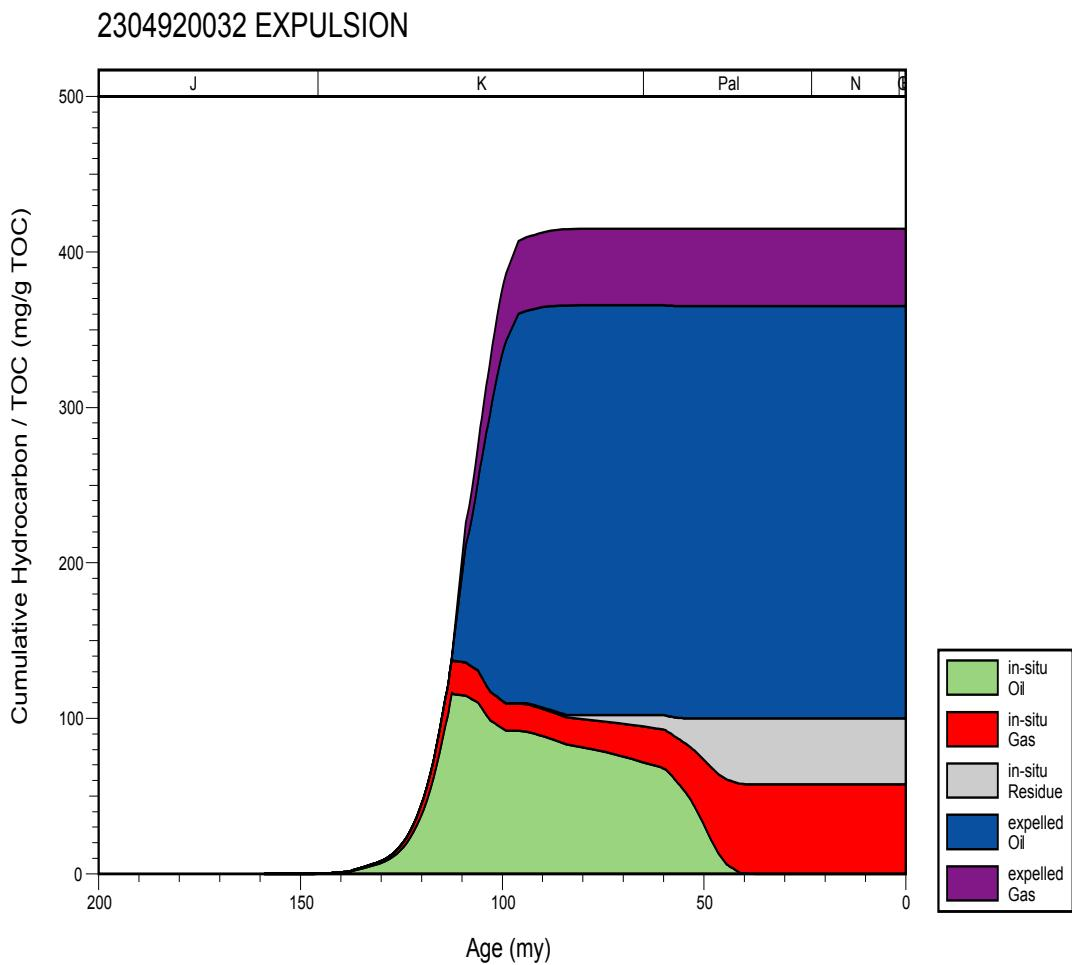
**Figure 59. Hydrocarbon expulsion plot for well 2304920032, Mississippi Interior Salt Basin.**
