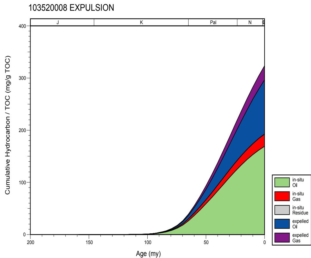
**Figure 65. Hydrocarbon expulsion plot for well 103520008, Conecuh Subbasin.**
