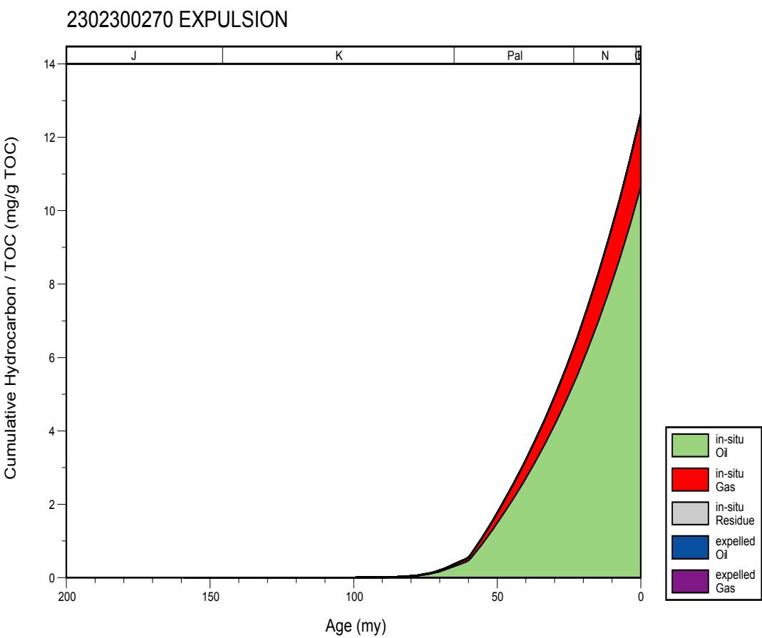
**Figure 60. Hydrocarbon expulsion plot for well 2302300270, Mississippi Interior Salt Basin.**
