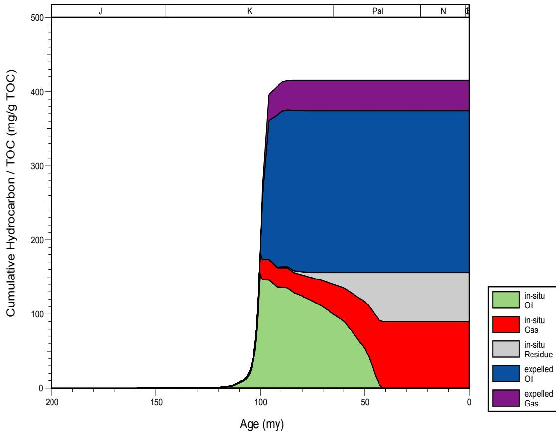
**Figure 61. Hydrocarbon expulsion plot for well 2311100069, Mississippi Interior Salt Basin.**
