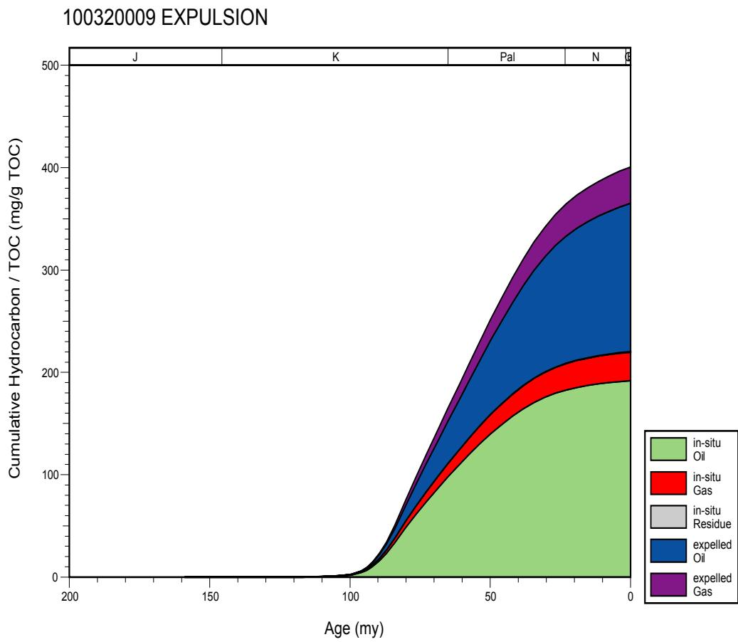
**Figure 67. Hydrocarbon expulsion plot for well 100320009, Conecuh Subbasin.**
