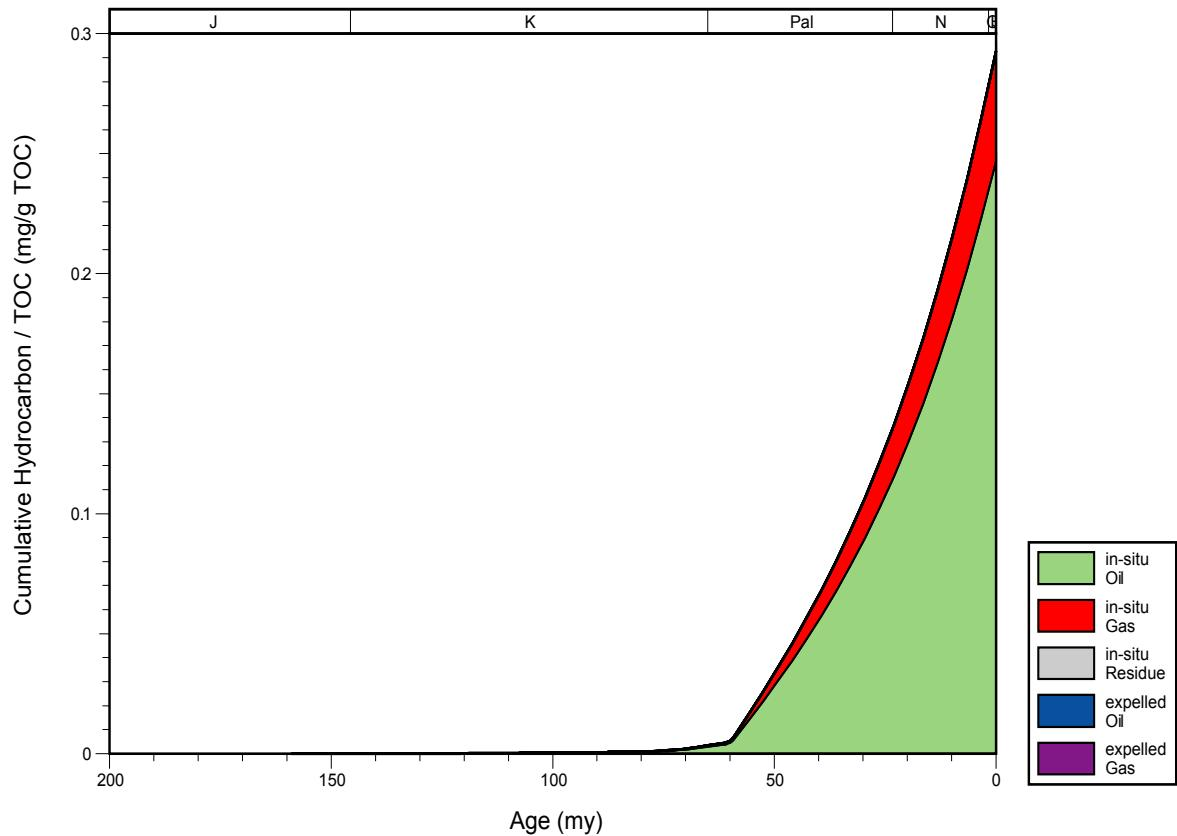
**Figure 58. Hydrocarbon expulsion plot for well 2308320011, Mississippi Interior Salt Basin.**
