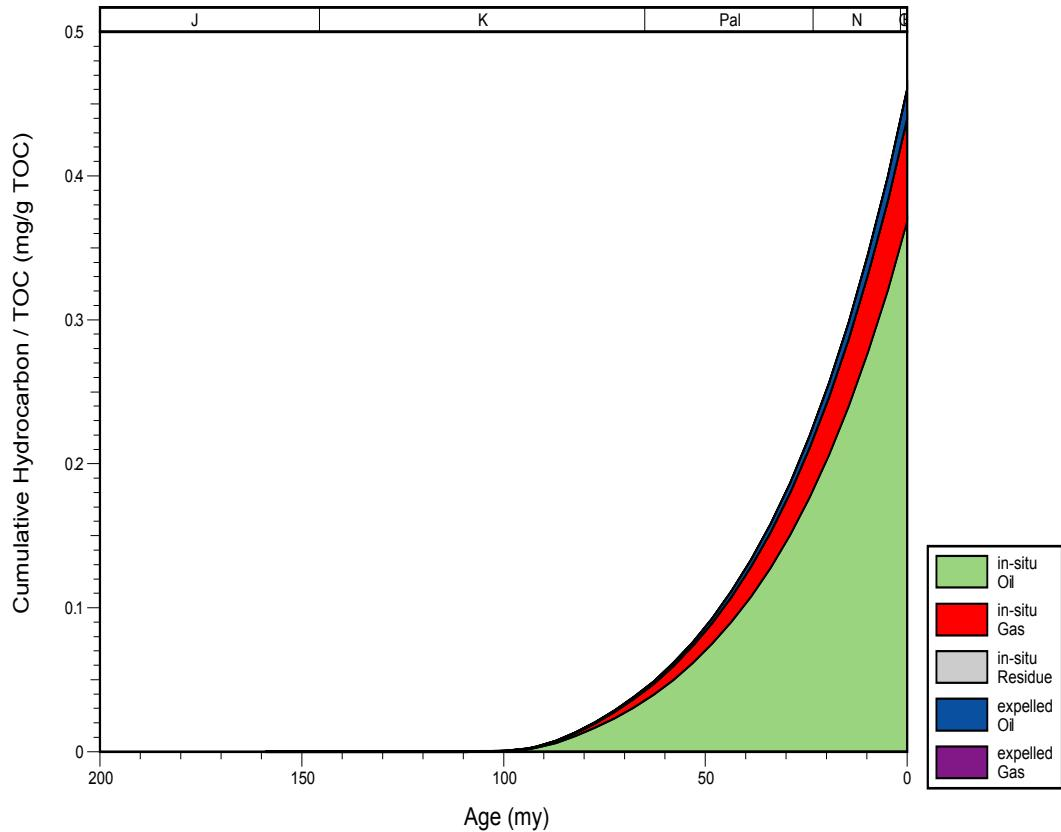
**Figure 62. Hydrocarbon expulsion plot for well 102520042, Manila Subbasin.**
