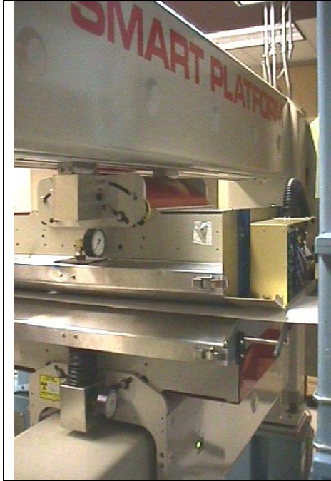
Side view of sensor during shake down trial on IPST web handler in winter-spring 2004. Note the sensor is attached to the ABB scanner head and scans the web thanks to the ABB scanner head like the other sensors do.
