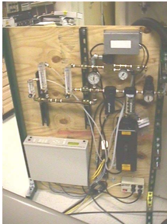
Auxiliary subsystem supplying power to motors and spinning mirror, purge air and cooling to sensor module, and air to the Bernoulli plate (web stabilizer)
