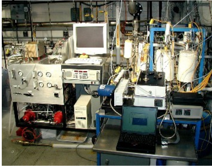
Figure 2. MPR Downstream Section, including reformate clean up and fuel cell test stand.
