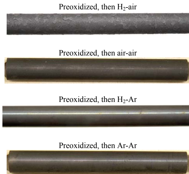
Fig. 5. Outer diameter scales after 100 hr exposures at 700°C.
