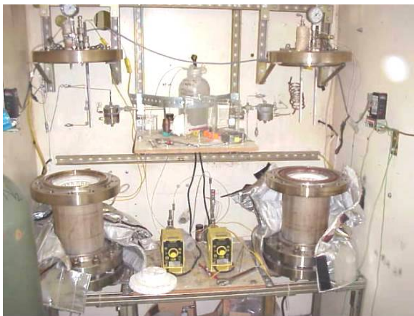
Figure 2-2. Interior of a high-pressure test cell containing two high-pressure aging reactors
