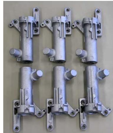
Figure 16: A 200T THT SLC casting cell and SiBloy® SSM castings produced.
