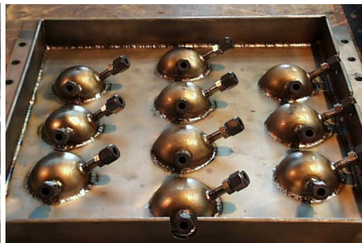
Rear view of dimpled plates #3 and #5 with gas injectors installed
