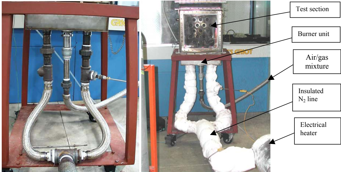
Figure 24. Modified Rig with Nitrogen Supply System
