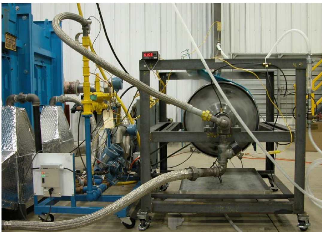
Figure 31. The GFD Test Rig Equipped with Air/Gas Supply and Heat Recuperation
