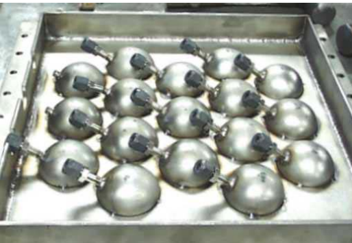
Rear view of dimpled plates #3 and #5 with gas injectors installed
