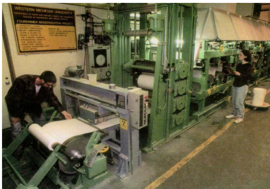
Figure 32. General View of WMU Pilot-Scale Paper Machine
