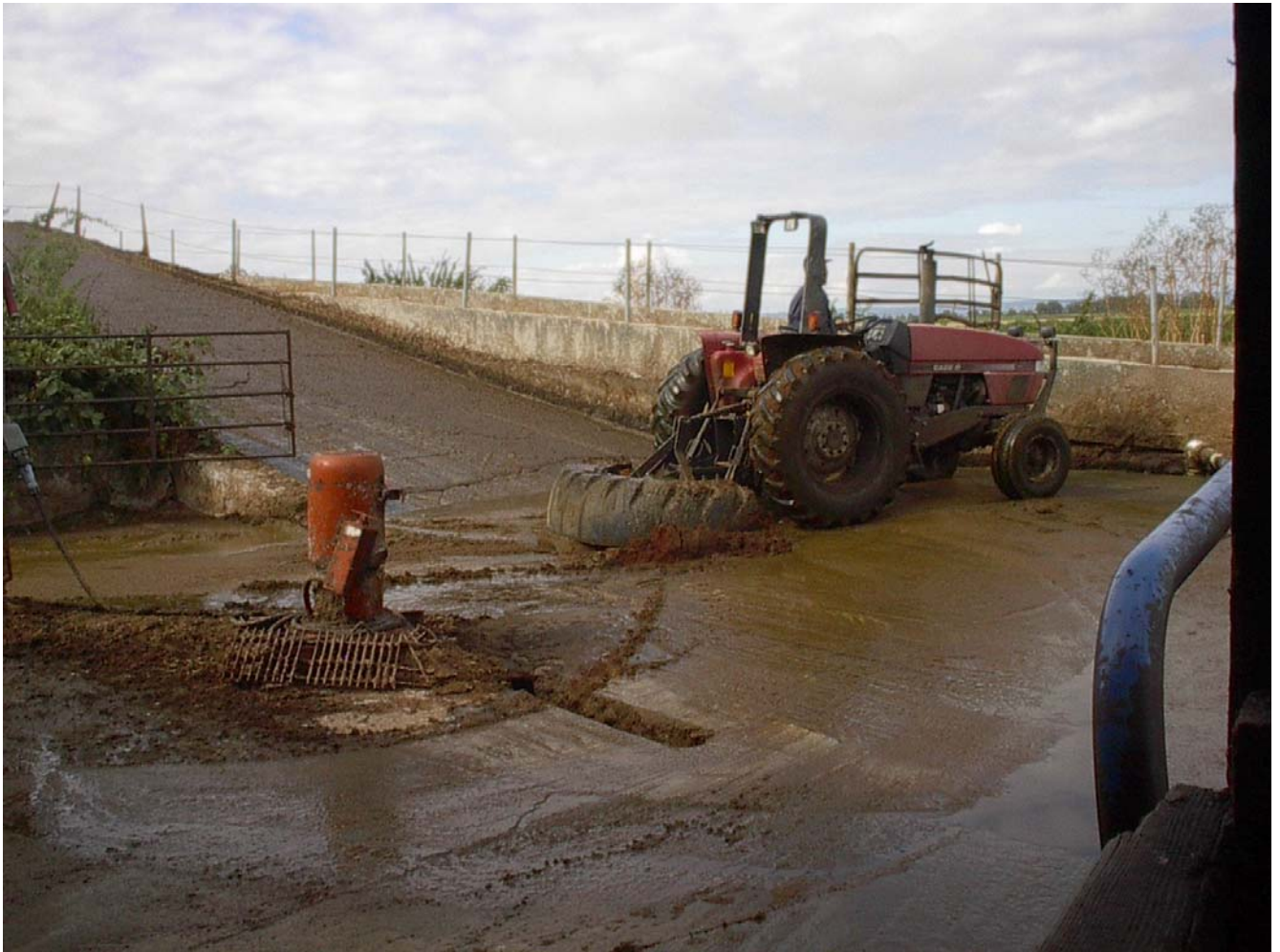
Figure 4. Typical Rubber Tire Scraped Manure Collection
