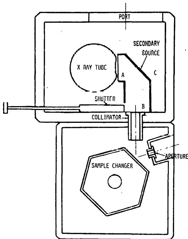
FIG. 1.--Cross sectional view (along the optical path) of the x-ray spectrometer.
