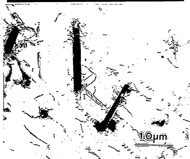
Figure 11: Transmission electron micrographs showing the two intragranular M_7C_3 carbide morphologies (globular and faceted) observed in the samples final-annealed at 1024°C for 1h.
