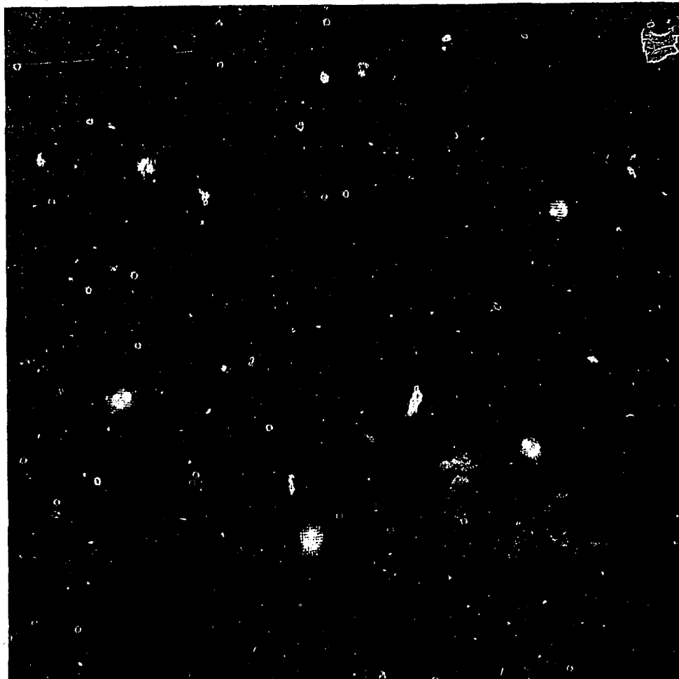
Fig. 2.21. LEED pattern from epitaxially grown Au (111) crystal at a primary beam energy of 54 eV.
